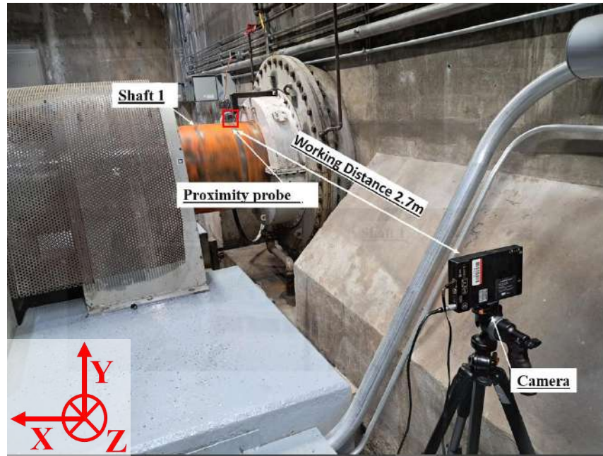
Figure 117: Experiment Setup for Shaft 1 in Y-Direction
