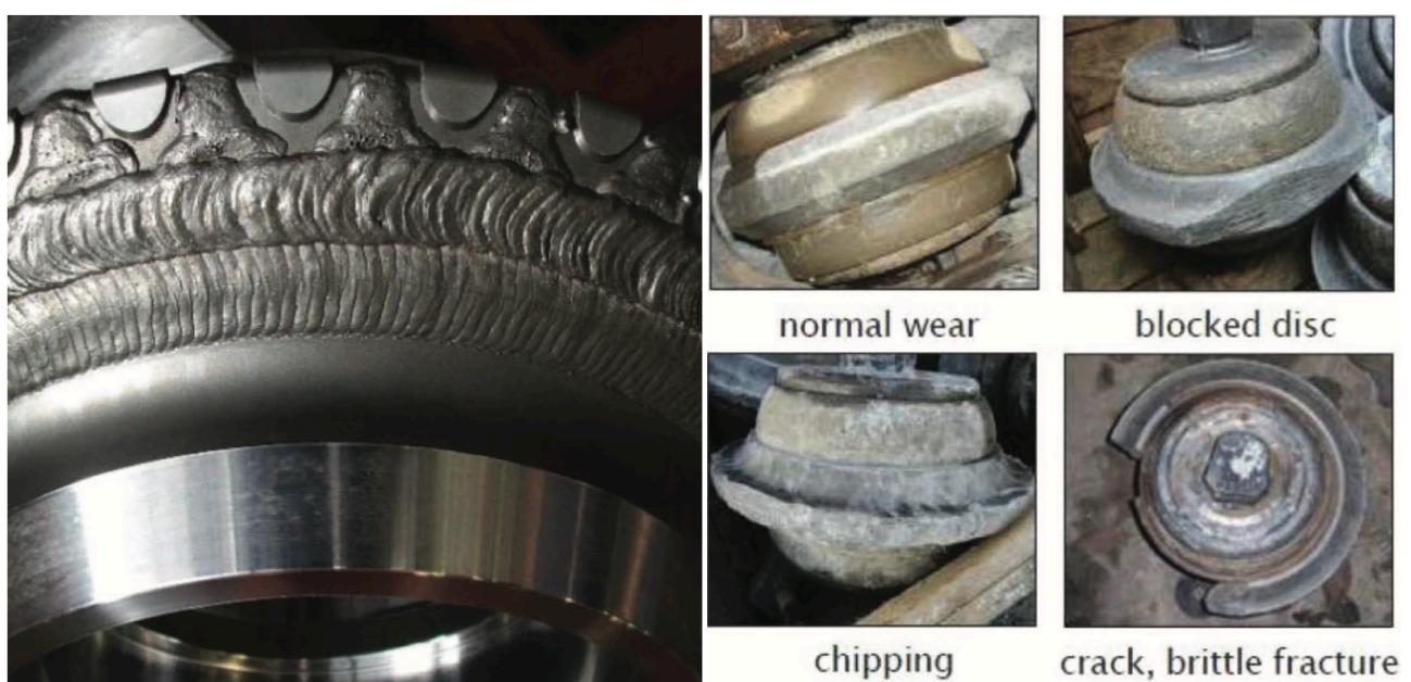
Figure 12: Cutter with tungsten carbide inserts, left. Cutter wear examples, right. Adapted from P. Grasso et al. (2023), figures 2.34 and 2.35
