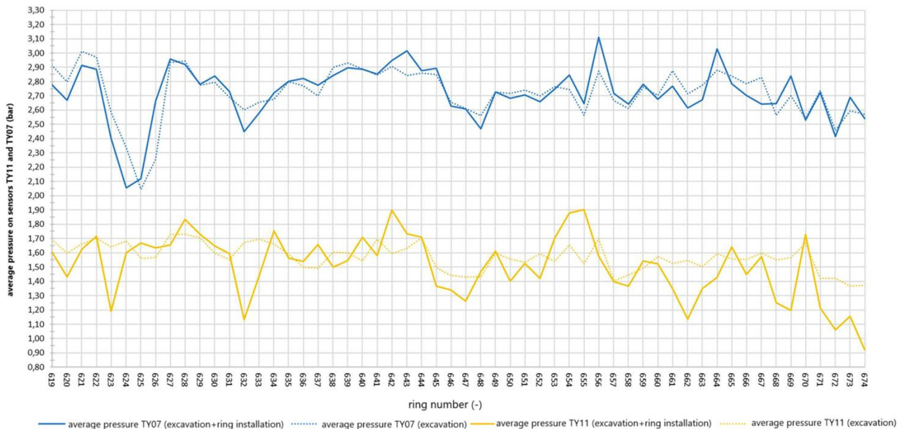
Figure 5.22 Face pressure: comparison between TY06 and TY11 sensors (Report, 2024)
