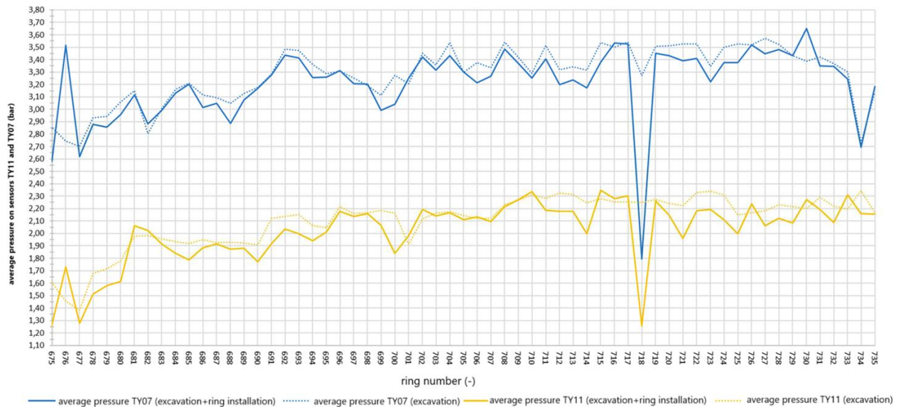
Figure 5.31 Face pressure: comparison between TY06 and TY11 sensors (Report, 2024)
