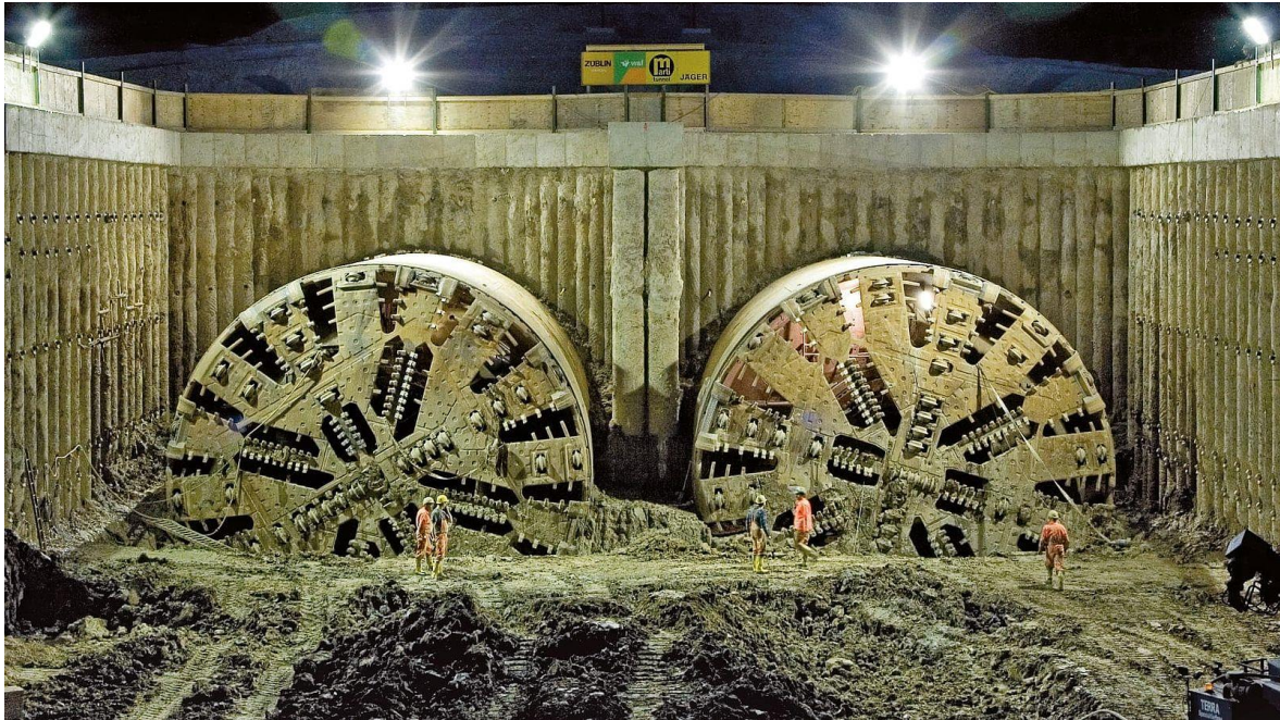
Figure 1.5 EPB Front view (Herrenknecht, 2025)
