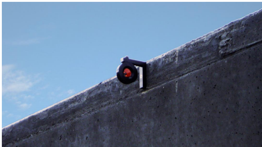
Figure 4.3 Example of an optical survey target (Sisgeo)
