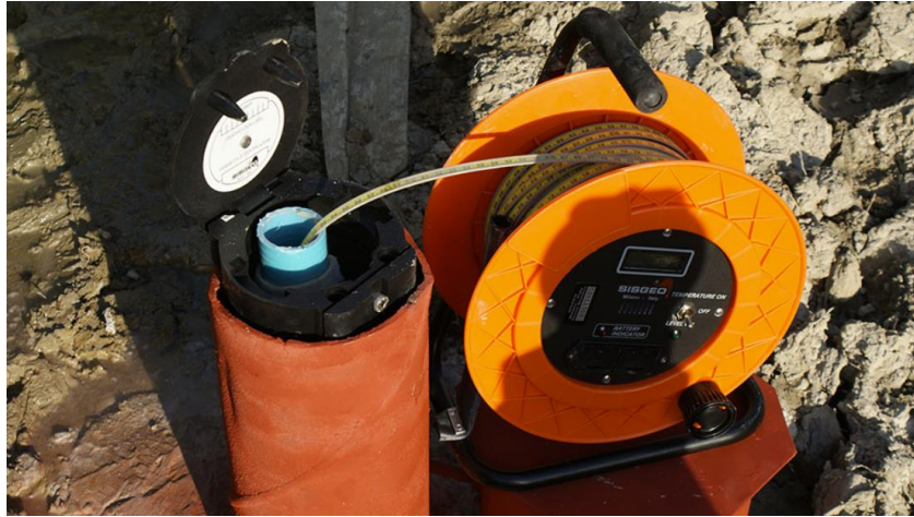
Figure 4.7 Open tube piezometers (Sisgeo)
