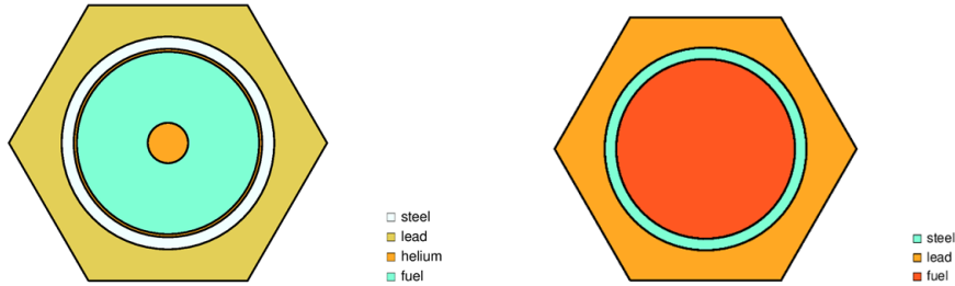
Figure 4.5: Heterogeneous fuel cell model on the left and the homogeneous one right
