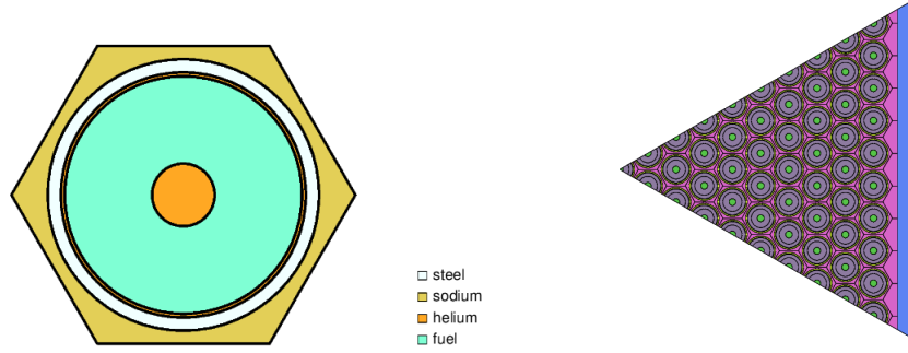
Figure 6.9: 3600\text{ MW}_{th} sodium-cooled fast reactor cell and fuel assembly
