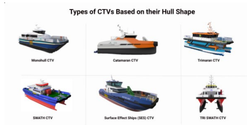
Figure 3. Crew Transfer Vessel (CTV) typologies
