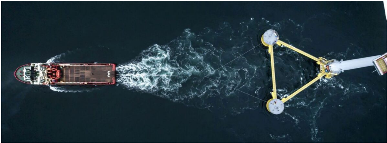
Figure 32: Floating turbine towed by an AHTS vessel
