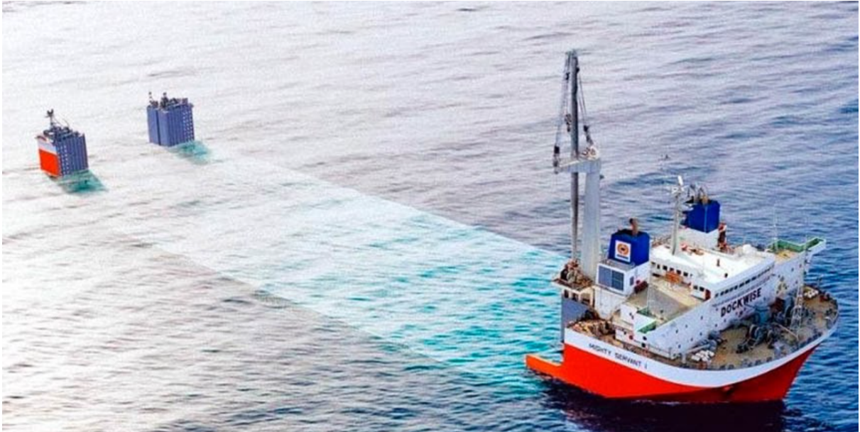
Figure 26: Semisubmersible vessel with submerged deck
