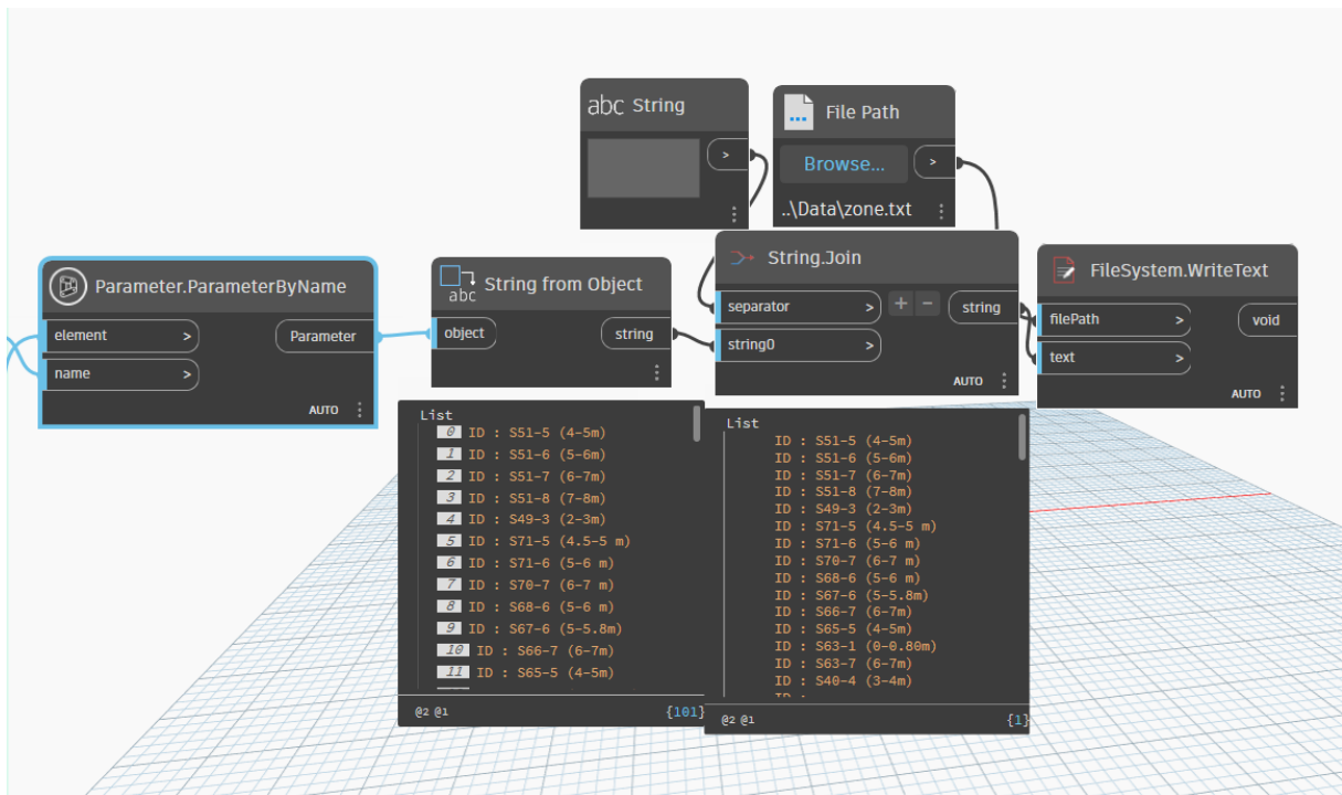
Figure 57. Script which saves the ID of the elements with dangerous concentration of pollutant.
