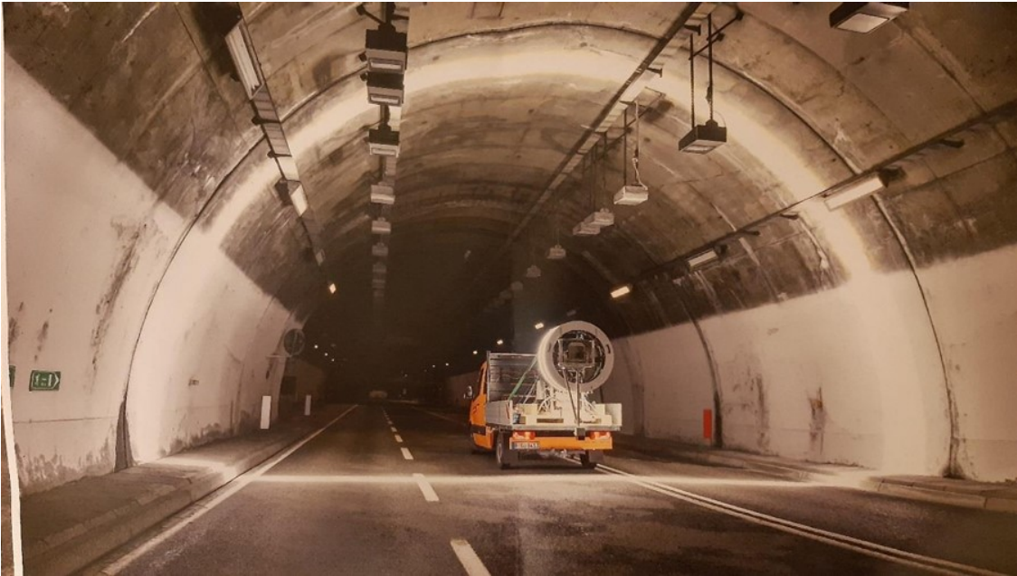
Figure 4.2: Vehicle equipped with Spacetec laser scanner collecting data in tunnels
