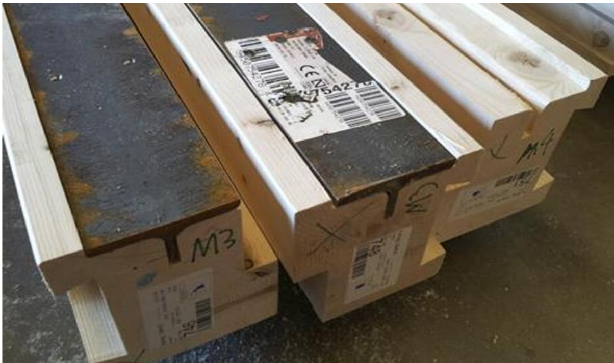
Figure 68 Steel and wood structural beams (Source: minivi.uadla.com)
