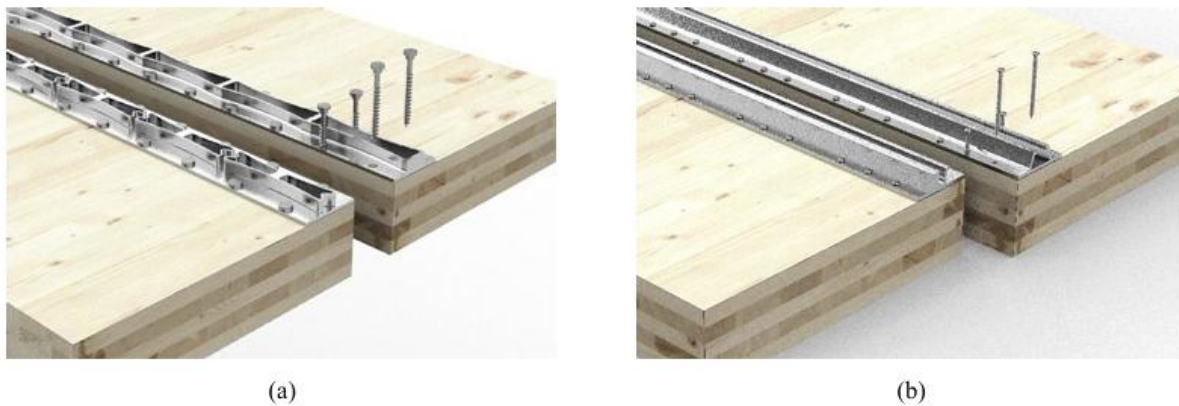
Figure 115 continuous connectors attached on the CLT panels using fasteners: (a) shear connectors, (b) tensile connectors [71]
