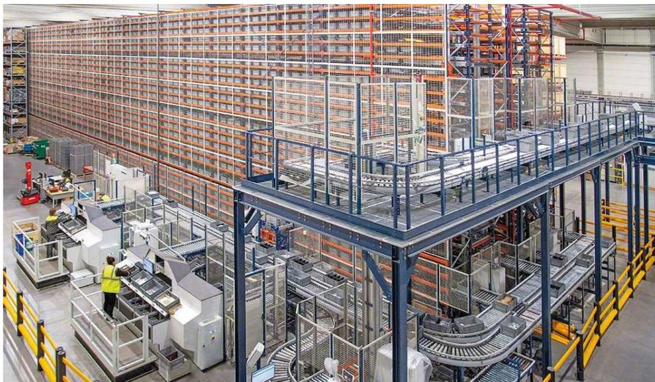
*Figure 4: Automatic storage system, Source [4]*
