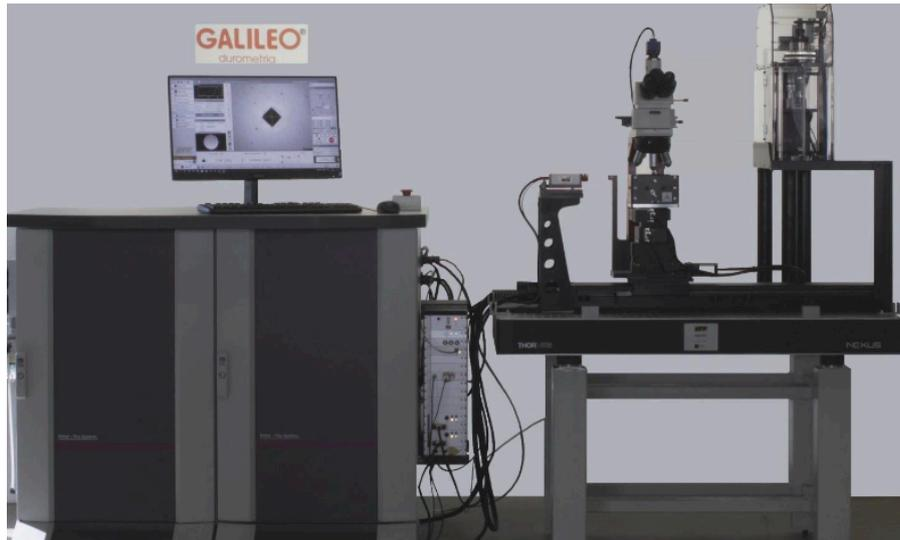
*Figura 10: MHSM, Micro Hardness Standardization Machine
