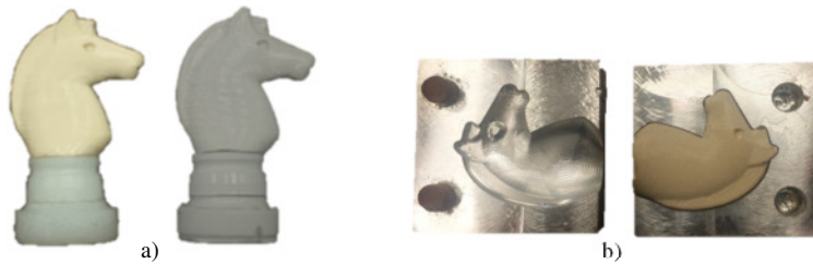
Figure 7. Knight quality issues a) Colour difference b) Fixture for hole drilling.
