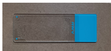
Fig. 2.2 Top view of the sample. A microscope glass slide (VWR) with dimensions 75 x 25 \text{mm}^2 and an cover slip (Epredia) with dimensions 55 x 25 \text{mm}^2 placed on top of it. A droplet of Paramecia between them. Scotch tape height of 50 \mu\text{m} .
