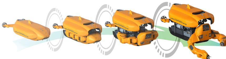
**Figure 1.3:** Shape-shifting AUV AQUANAUT
