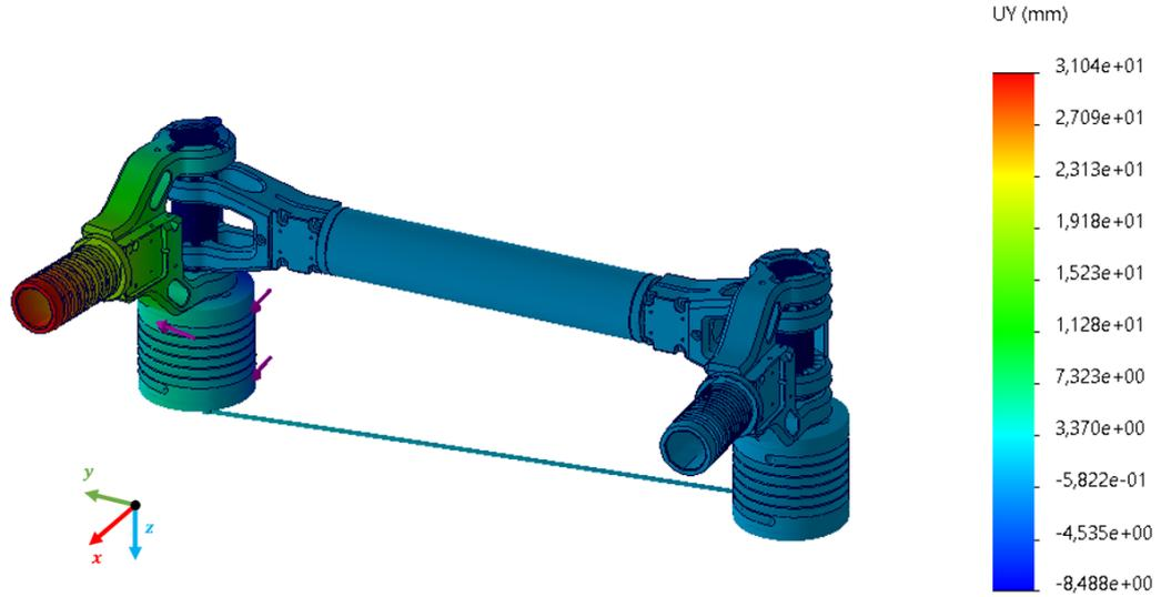
**Figure 7.7:** Experimental parameters - displacement along the  $y$  direction [mm]
