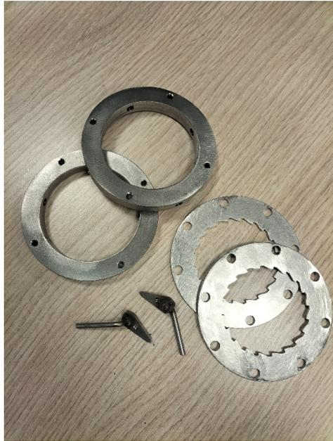
**Figure 9.1:** Metal components of the pulleys
