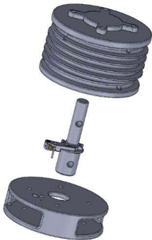
**Figure 8.1:** Exploded view of the pulley
