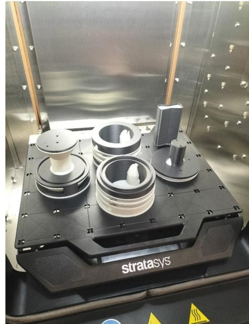
**Figure 9.2:** 3D printing of the components of the pulleys
