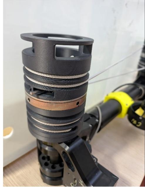
**Figure 9.4:** *Pulley A* assembled on RUVIFIST for the final test
