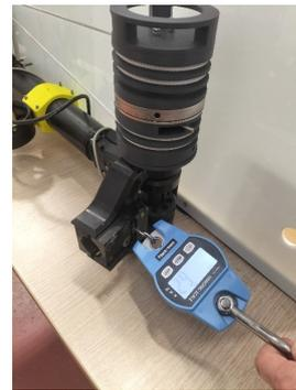
**Figure 7.2:** Load cell simulating the external disturbance  $F_d$
