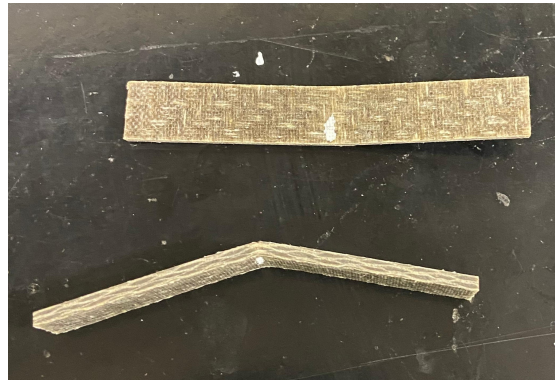
Figure 3.14: Two tested bending specimen
