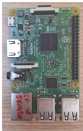
Figure 5.3: Raspberry PI 3rd generation
