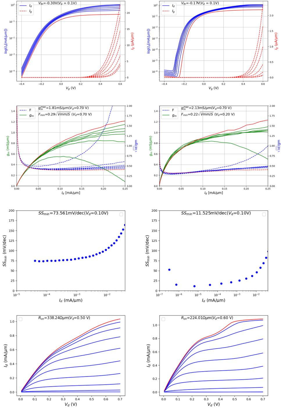
**Figure A.12:** HEMT DC: sample *SA2*, *EpiB-0.6nm*, for  $L_g = 10$  nm and  $w = 10$   $\mu\text{m}$  at RT (left) and 4K (right)
