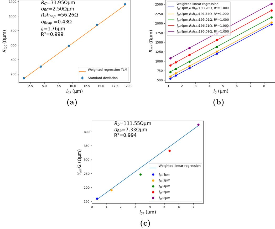
**Figure 4.6:** Resistive parameters extraction for EpiB-1nm at RT
