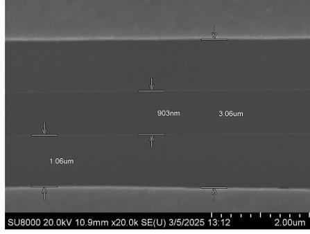
**Figure 4.1:** SEM image of recess-TLM for design lengths of  $l_g = 0.6 \mu\text{m}$  and  $l_{gs} = 2 \mu\text{m}$
