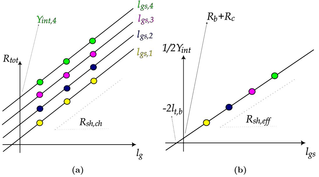
**Figure 2.6:** a) Schematic plot for the extraction of  $R_{sh,ch}$  and the y-intercepts, b) Schematic plot for the extraction of  $R_{sh,eff}$  and  $R_b$
