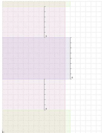
**Figure 3.2:** Example of recessed TLM design,  $l_g = 8 \mu\text{m}$ ,  $l_{gs} = 6 \mu\text{m}$
