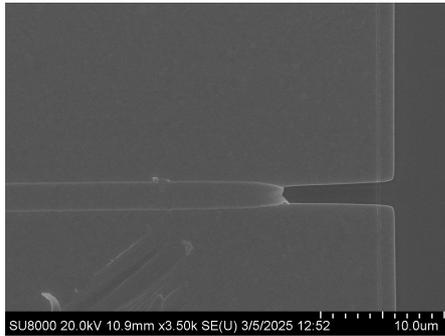
**Figure 4.3:** SEM image of shorted recessed TLM for design lengths of  $l_g = 0.6$   $\mu\text{m}$  and  $l_{gs} = 14$   $\mu\text{m}$
