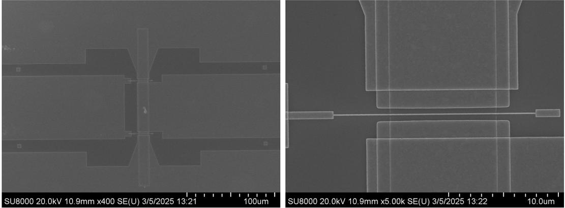
**Figure 4.4:** SEM images of a working HEMT with  $L_g = 100$  nm
