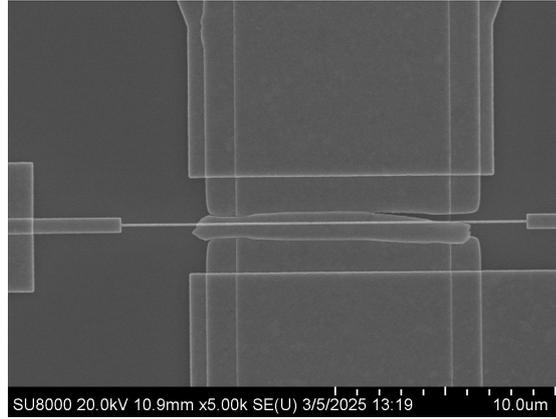
**Figure 4.5:** SEM images of a HEMT with non-completed gate lift-off, EpiB-1nm  $L_g = 100$  nm
