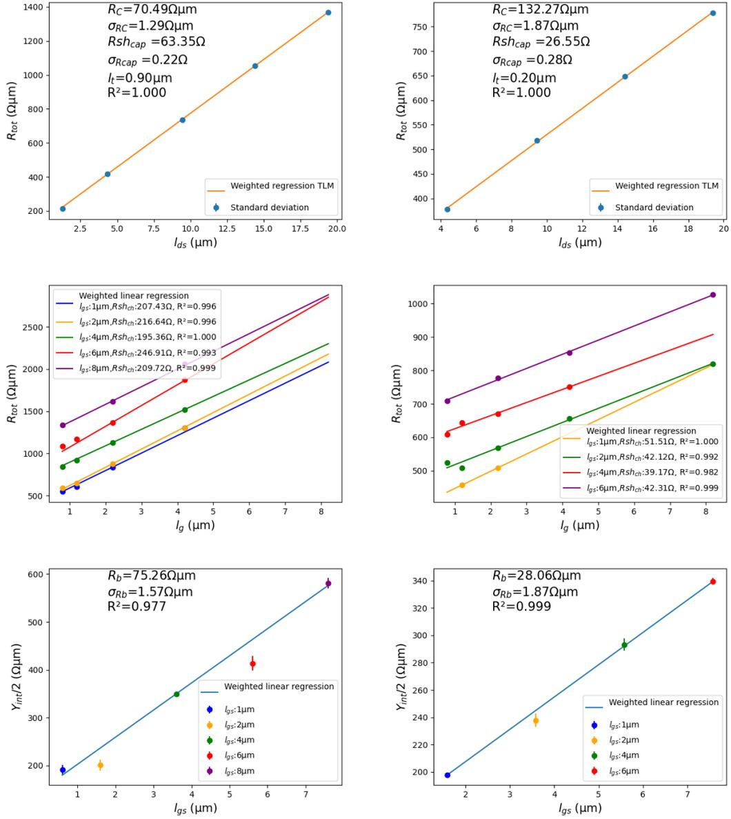
Figure A.3: TLM, sample SA1, *EpiA-10nm*, RT (left), 4 K (right)
