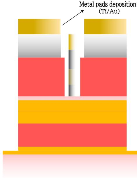
**Figure 3.9:** Metal pads deposition
