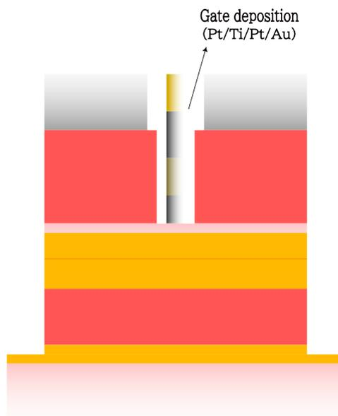
**Figure 3.8:** Gate deposition
