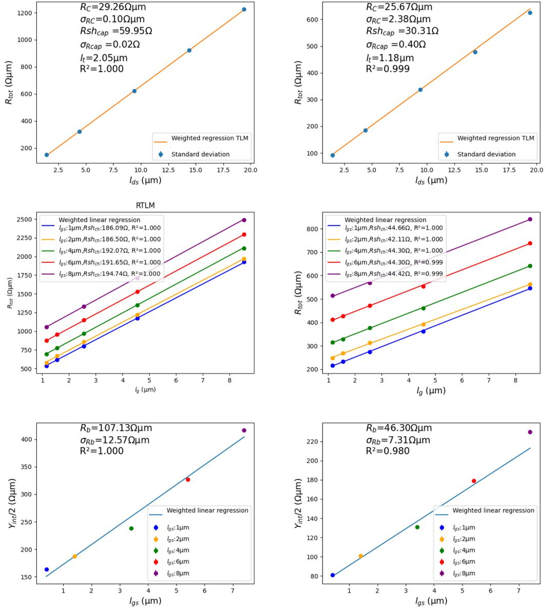
Figure A.9: TLM, sample *SB2*, *EpiB-3nm*, RT (left), 4 K (right)
