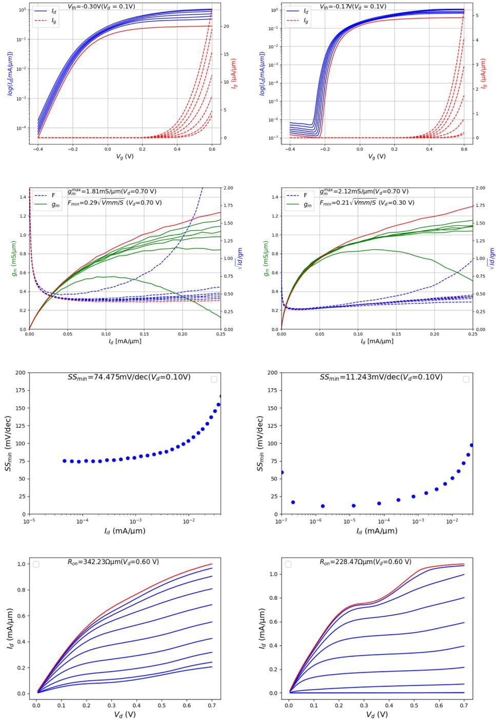
**Figure A.13:** HEMT DC: sample *SA2*, *EpiB-2nm*, for  $L_g = 10$  nm and  $w = 10$   $\mu\text{m}$  at RT (left) and 4 K (right)
