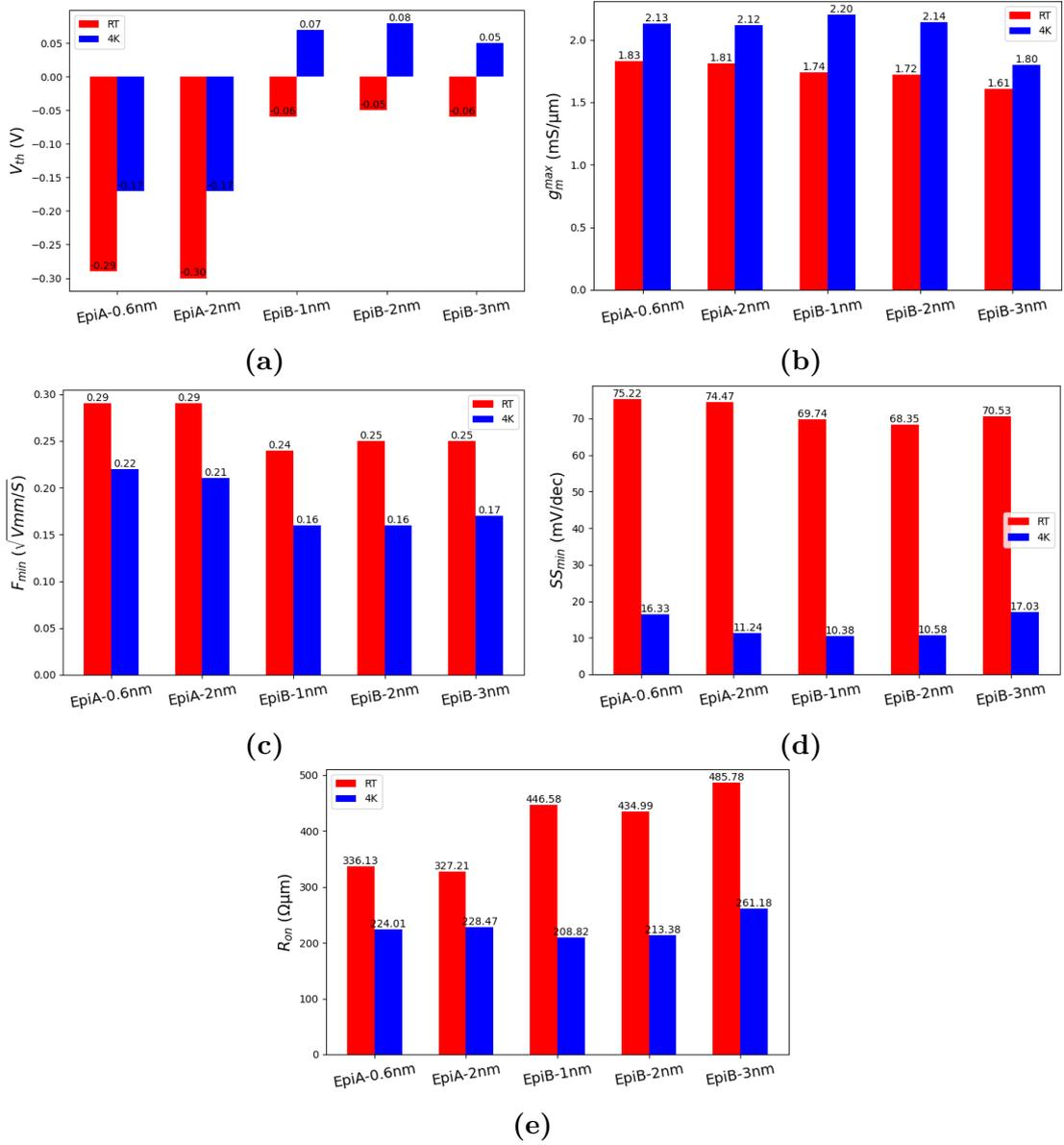
**Figure 4.11:** Variation of HEMTs metrics among the fabricated devices for  $L_g = 40$  nm and  $w = 10$   $\mu$ m
