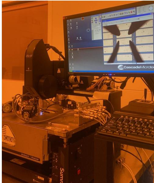
**Figure 3.10:** Probe station used for RT measurements
