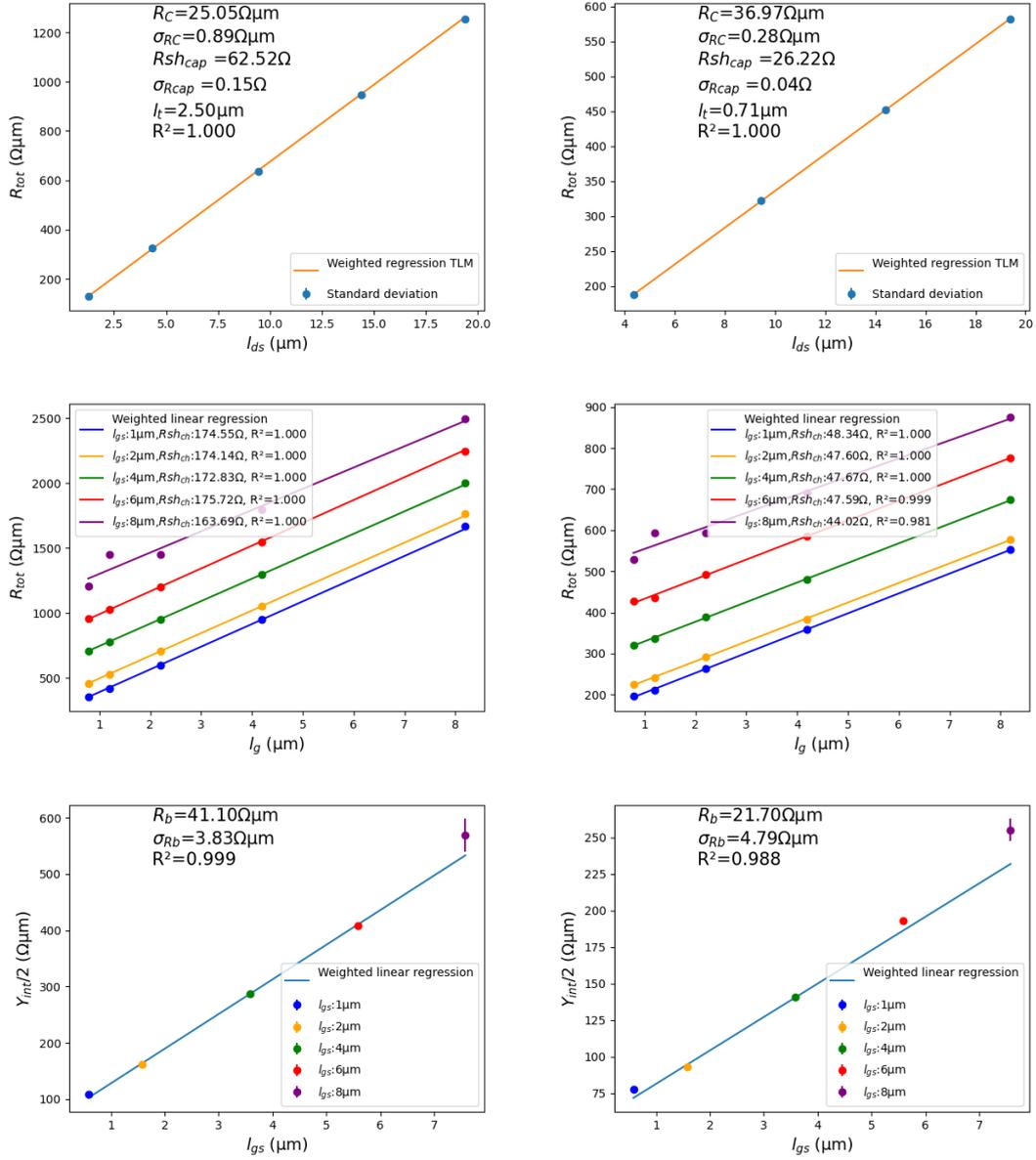
Figure A.1: TLM, sample SA1, *EpiA-3nm*, RT (left), 4 K (right)
