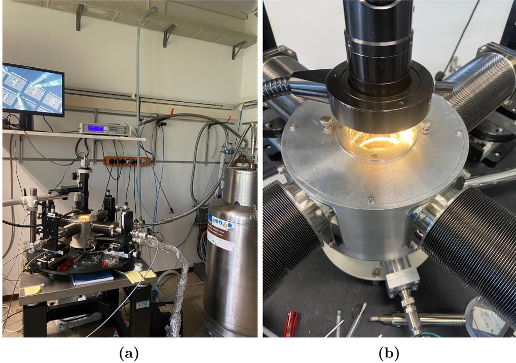
**Figure 3.11:** a) Cryogenic probe station with helium pump, b) zoom on the chuck of the cryogenic probe station
