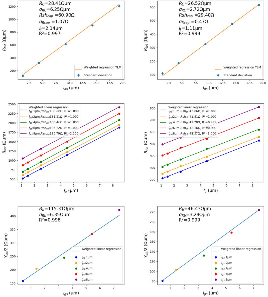
Figure A.10: TLM, sample *SB3*, *EpiB-2nm*, RT (left), 4 K (right)
