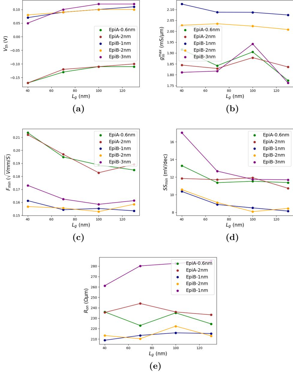
**Figure 4.13:** Dependence of HEMTs metrics on gate length for  $w = 10 \mu\text{m}$  at 4 K
