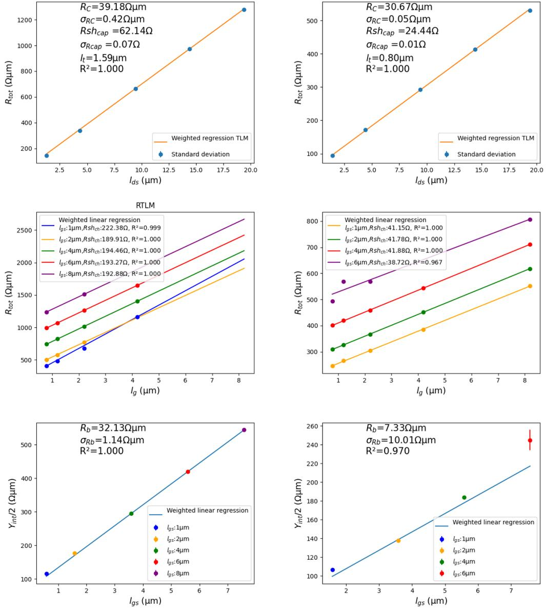
Figure A.2: TLM, sample SA1, *EpiA-6nm*, RT (left), 4 K (right)
