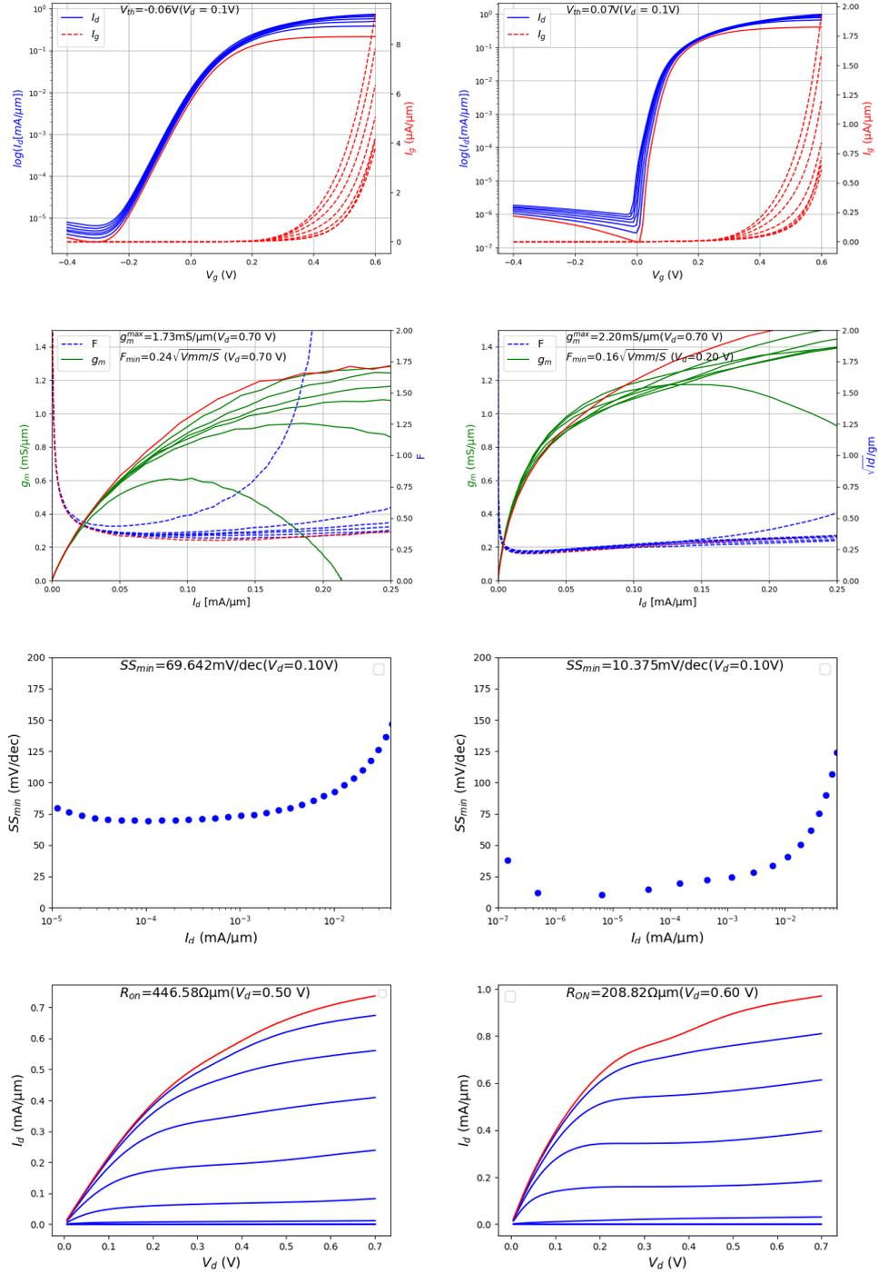
Figure A.14: HEMT DC: sample SB1, EpiB-1nm, for  $L_g = 10$  nm and  $w = 10$   $\mu m$  at RT (left) and 4 K (right)
