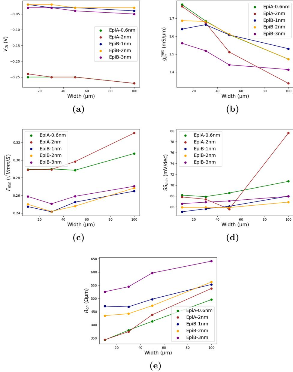
**Figure 4.14:** Dependence of HEMTs metrics on device width for  $L_g = 40$  nm at RT
