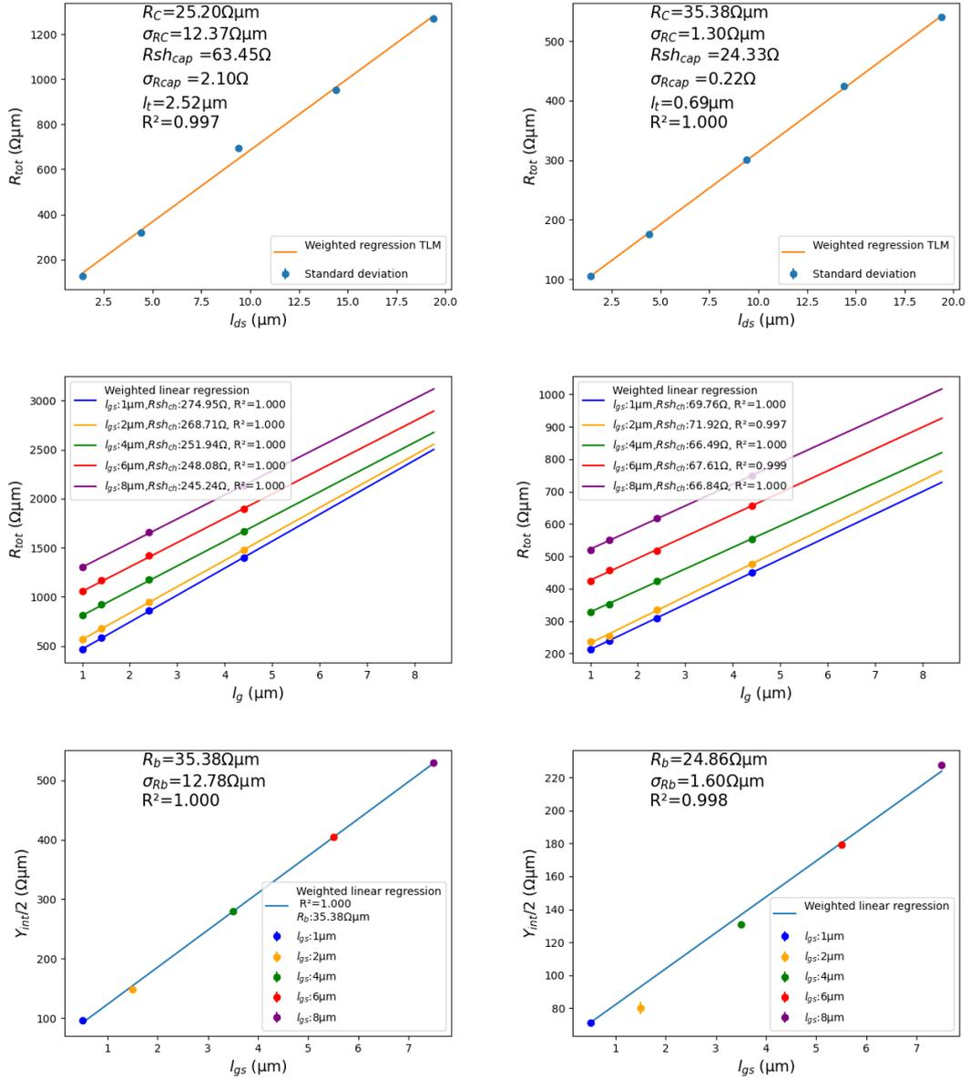
Figure A.7: TLM, sample SA2, *EpiA-3nm*, RT (left), 4 K (right)
