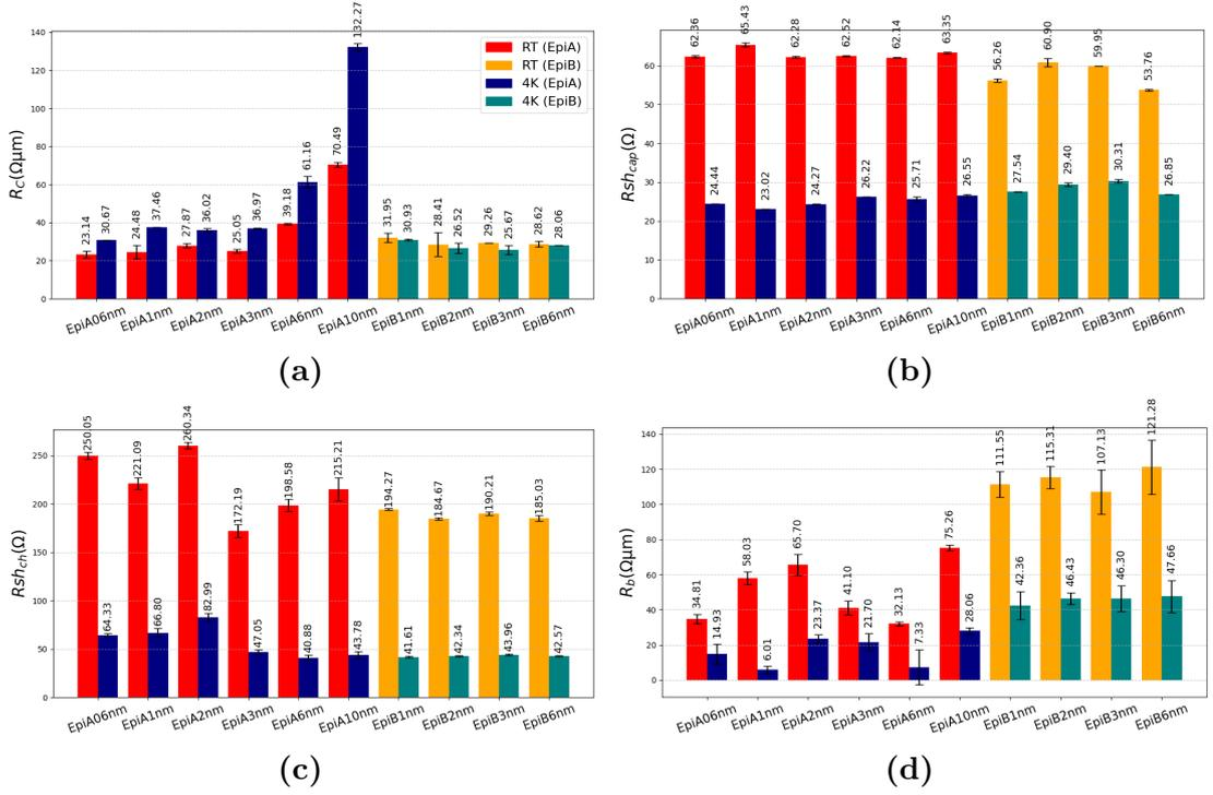
**Figure 4.10:** Resistive components variation among the fabricated devices
