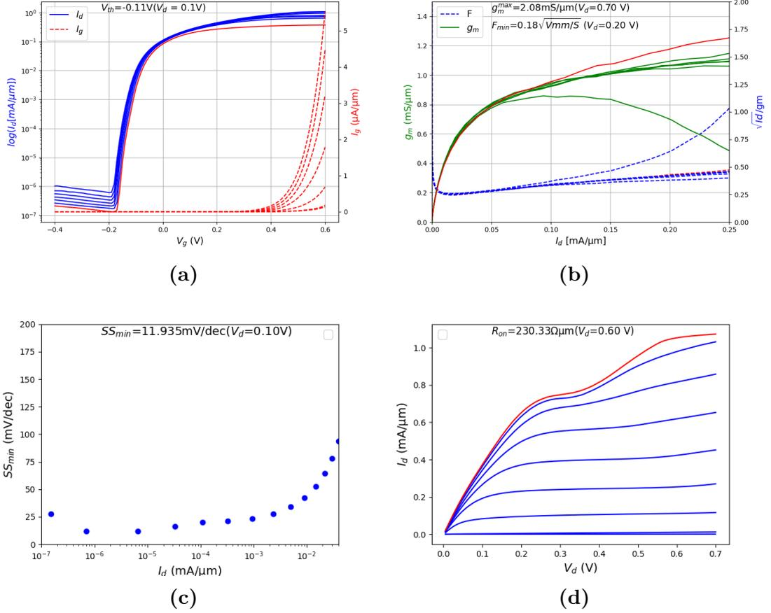
**Figure 4.9:** HEMTs DC characterization for EpiA-2nm  $L_g = 100\text{ nm}$ ,  $w = 10\ \mu\text{m}$  at 4 K
