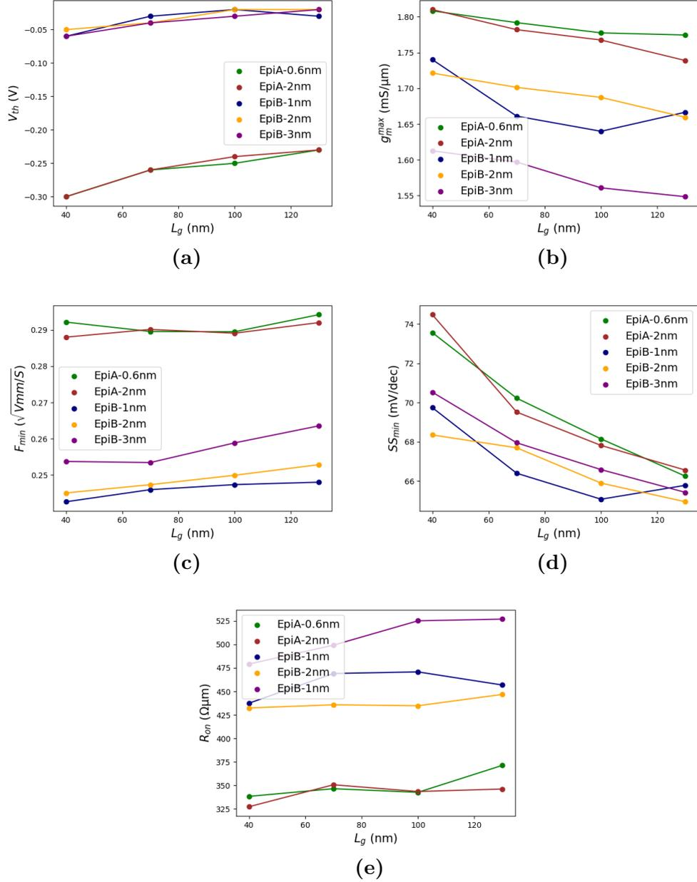
**Figure 4.12:** Dependence of HEMTs metrics on gate length for  $w = 10 \mu\text{m}$  at RT
