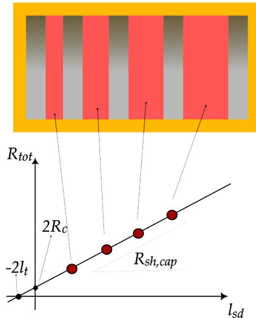
**Figure 2.4:** Schematic plot for the extraction of resistive components in non-recessed TLM structure
