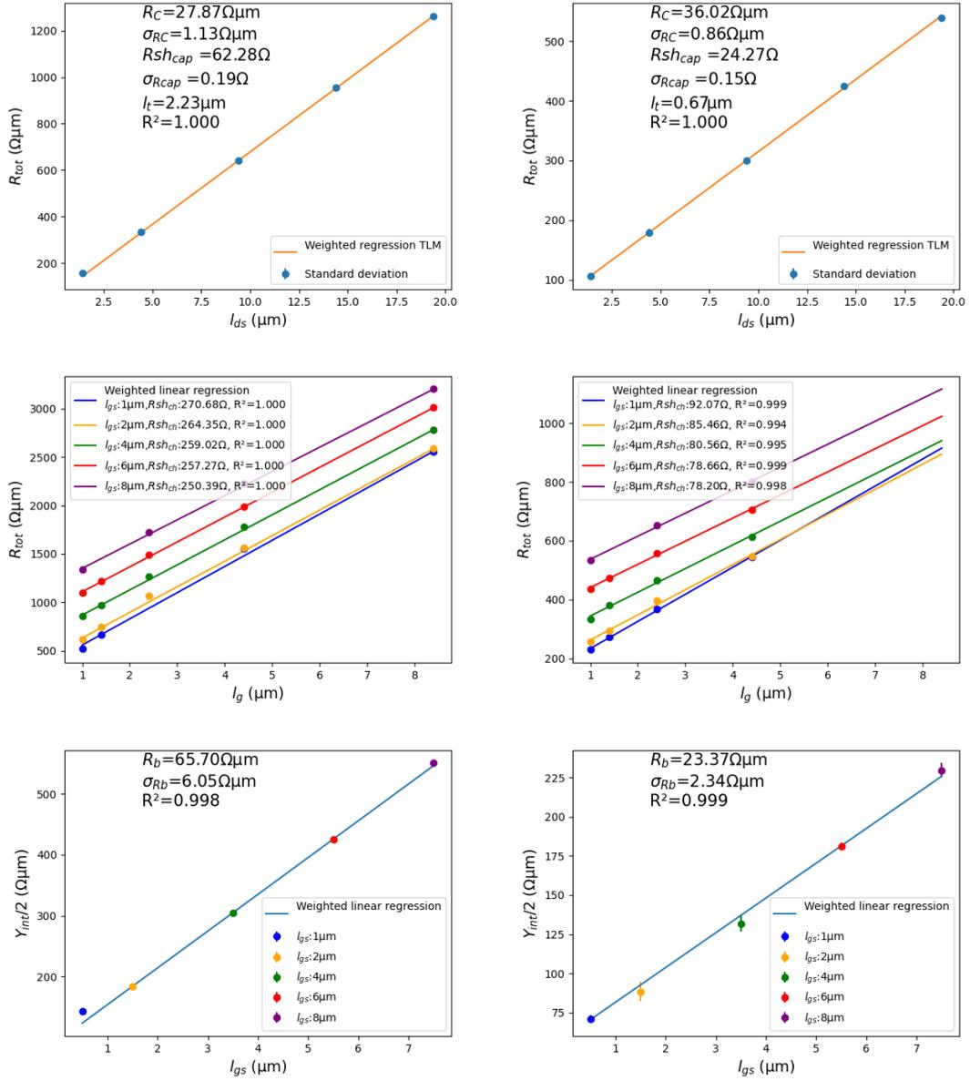
Figure A.6: TLM, sample SA2, *EpiA-2nm*, RT (left), 4 K (right)
