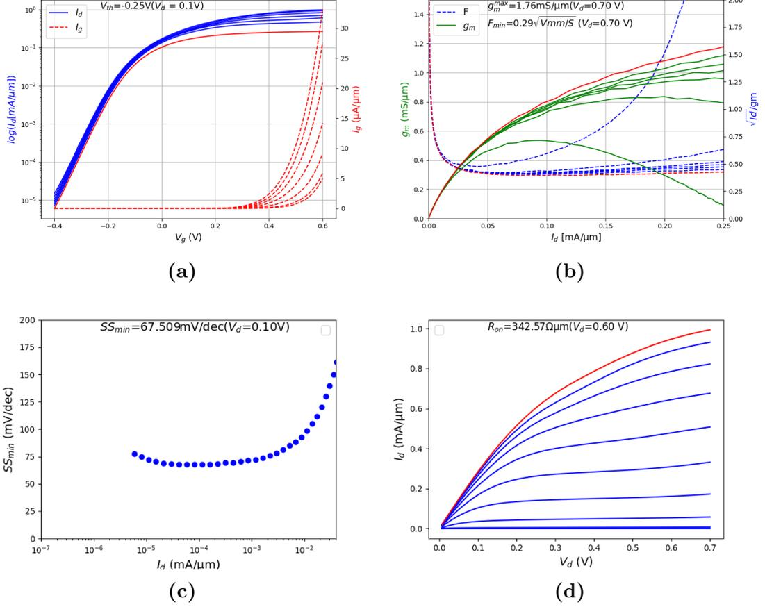
**Figure 4.8:** HEMTs DC characterization for EpiA-2nm  $L_g = 100$  nm,  $w = 10$   $\mu\text{m}$  at RT
