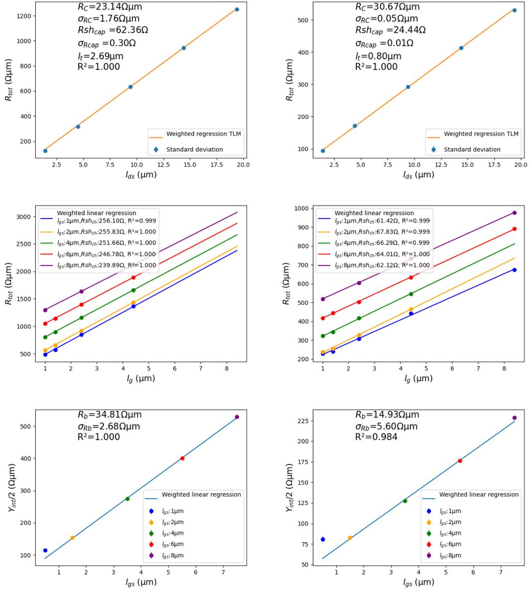
Figure A.4: TLM, sample SA2, *EpiA-0.6nm*, RT (left), 4 K (right)
