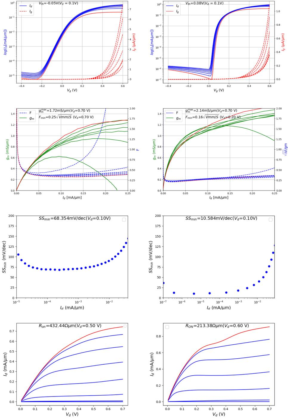
**Figure A.15:** HEMT DC: sample *SB3*, *EpiB-2nm*, for  $L_g = 10$  nm and  $w = 10$   $\mu\text{m}$  at RT (left) and 4 K (right)
