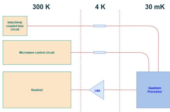
**Figure 1.1:** Quantum computer control system schematic
