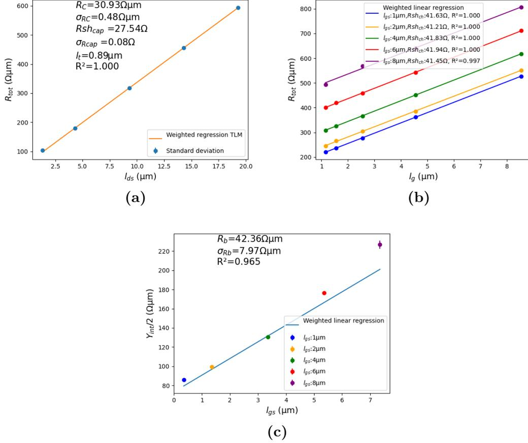
**Figure 4.7:** Resistive parameters extraction for EpiB-1nm at 4K
