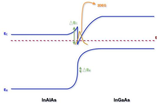
**Figure 2.1:** Simplified band diagram of an InGaAs HEMT
