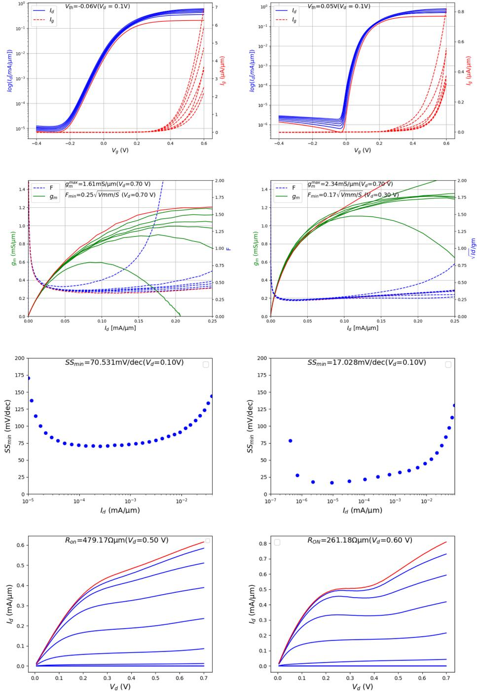
**Figure A.16:** HEMT DC: sample *SB2*, *EpiB-3nm*, for  $L_g = 10$  nm and  $w = 10$   $\mu\text{m}$  at RT (left) and 4 K (right)
