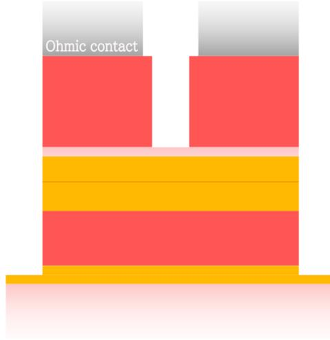
**Figure 3.7:** Ohmic contact deposition
