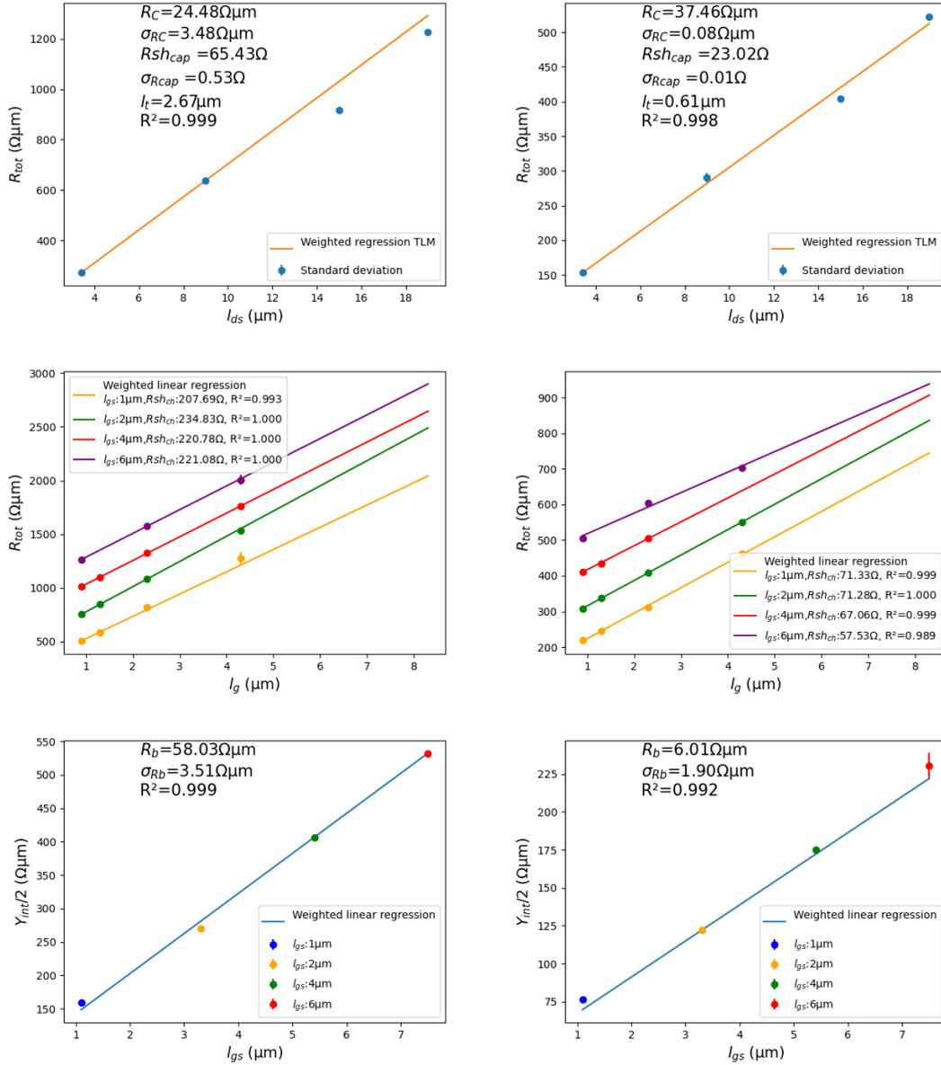
Figure A.5: TLM, sample SA2, *EpiA-1nm*, RT (left), 4 K (right)
