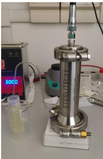
Figure 7: Dead-end filtration set-up.
