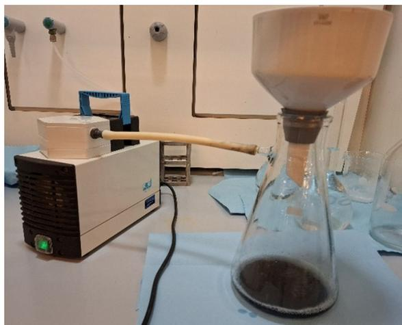
Figure 17: System used for the vacuum-assisted coating of  $NiFeCo$  on the sintered nickel felt substrate, showing the vacuum pump and the Buchner funnel containing the filter.
