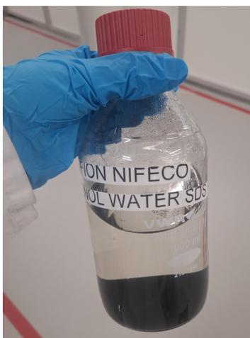
Figure 26: Dispersion of  $NiFeCo$  with Nafion, 2-propanol and SDS used for the Ultraturrax-assisted coating method. The nanoparticles tended to precipitate at the bottom of the container.
