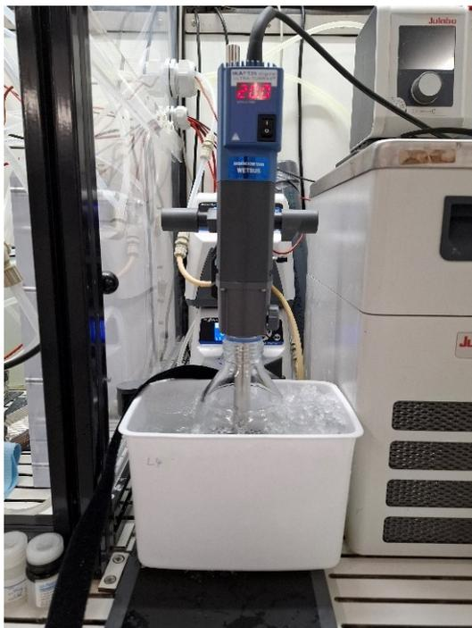
Figure 16: System used for the Ultraturrax-assisted coating of sintered nickel felt with *NiFeCo* electrocatalyst, showing the Ultraturrax at 20000rpm and the integrated ice bath.
