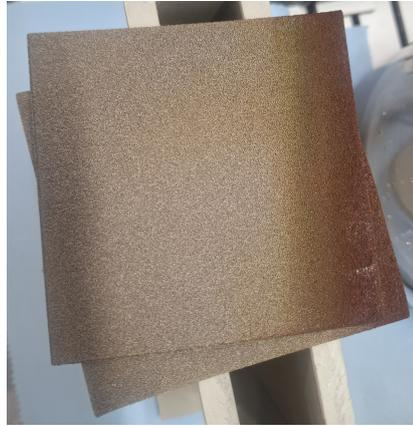
Figure 31: *Ni*-foam (10cm x 10cm) partially coated with *NiFeCo* (right side) using dip-coating. The partial coating, highlighted by the color change, that occurred was due the absence of oxygen due to sealing flat PP container with Parafilm tape. However, the presence of oxygen gas appeared essential for the electrochemical reactions to occur.
