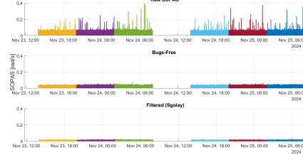
Figure 4.13: Effect of Removing Bugs and Applying Sgolay Filter on Six Circuit-2 Batches.
