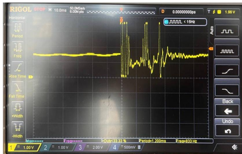
**Figure 4.15:** The single supply circuit's response to a signal with overvoltage
