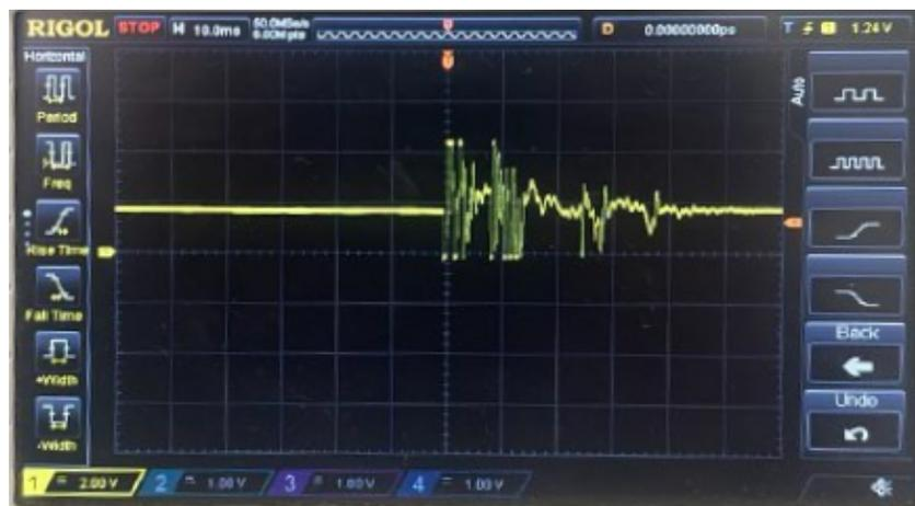
**Figure 4.11:** The dual-supply circuit's response to an overvoltage signal
