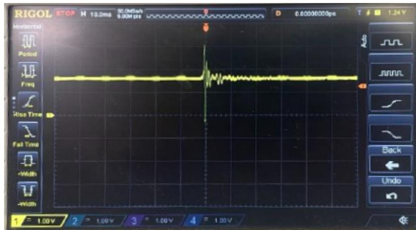
**Figure 4.10:** The dual-supply circuit's output to a typical PLB test as input
