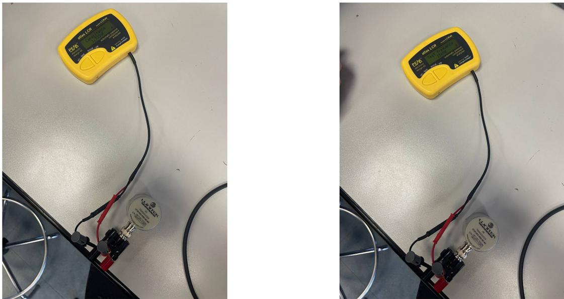
Figure 4.3: The AE sensor's capacitance at 15 kHz
