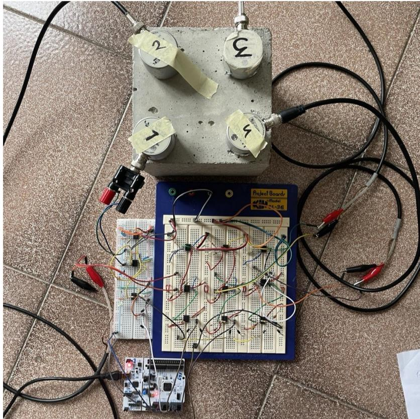
**Figure 5.2:** Test setup on concrete block
