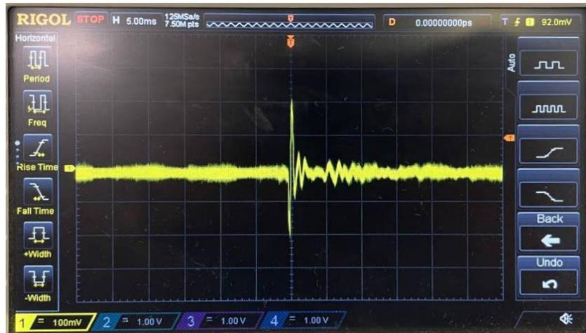
**Figure 4.7:** The charge amplifier circuit's output
