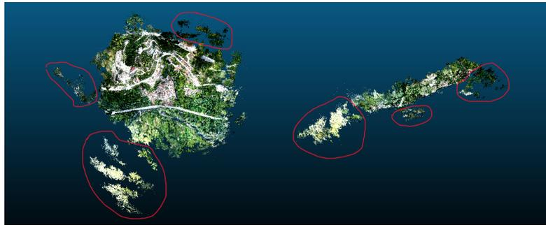
**Figure 4.6:** DN-Splatter point cloud, displayed in CloudCompare. On the left, the top view of the scene is shown, on the right the side view of the same scene. Outliers, circled in red, are highlighted.
