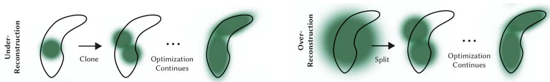
**Figure 3.4:** Adaptive density control of 3D gaussians
