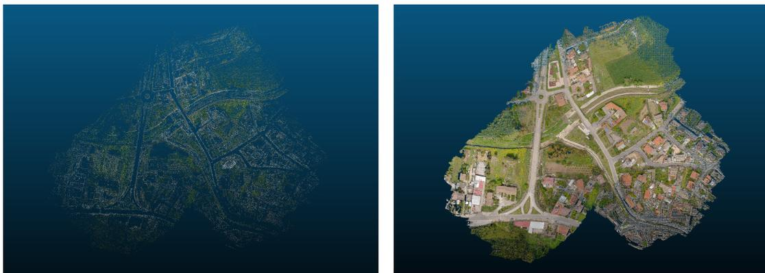
**Figure 2.5:** Sparse reconstruction (on the left) versus dense reconstruction (on the right) of the same urban environment: comparison of resulting point clouds obtained respectively with SfM and MVS technique.
