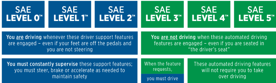
Figure 2.1: SAEJ3016 Levels of Driving Automation [5]
