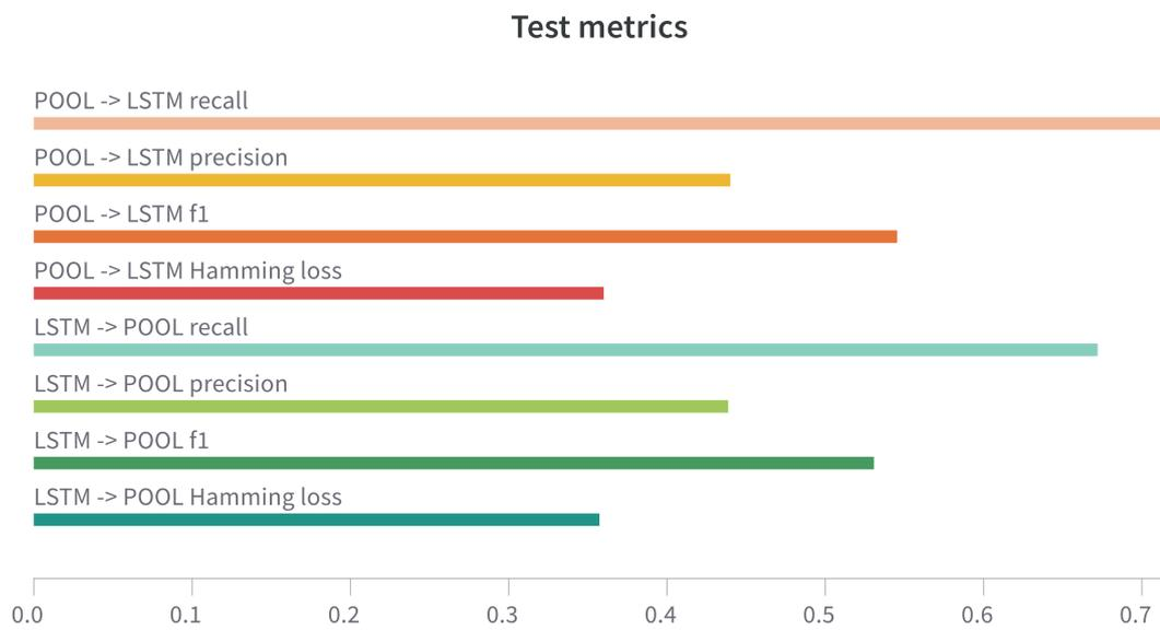
Figure 73: Test metrics for two different designs (pooling layer followed by bi-LSTM layer / bi-LSTM layer followed by pooling layer).
