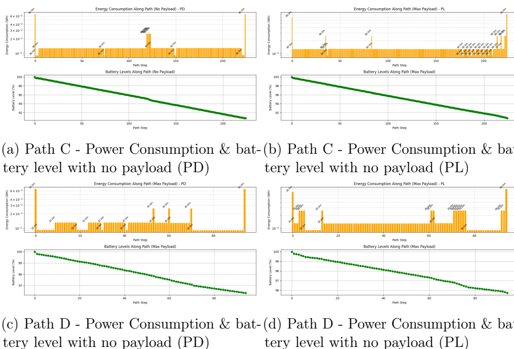
Figure 5.36: Power Consumption and battery level trends using Avata 2 along path C & D in small graph.
