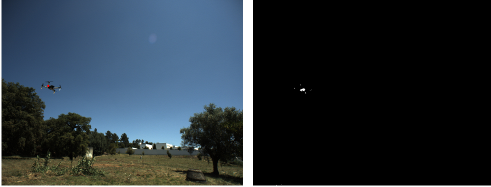
Figure 5.2: (a) Detected drone, marked with a red dot (b) The corresponding binary mask
