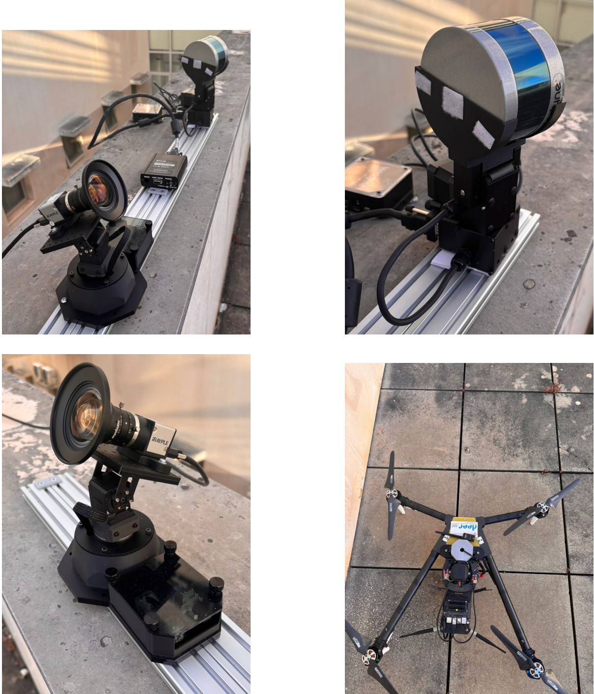
Figure 5.1: (a) Overall setup (b) Velodyne VLP16 on a PTU 46-17.5 (c) Camera on a PhantomX XL430 (d) Drone
