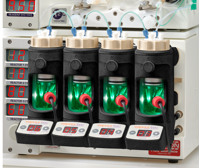
Figure 3.2: A chemical Continuous Stirred Tank Reactor (CSTR)
