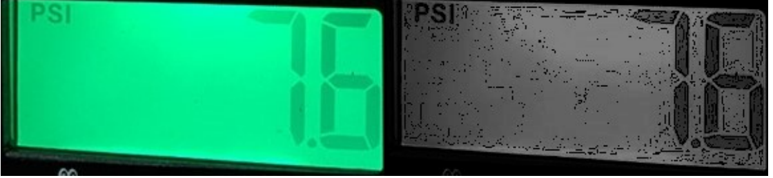
Figure 3.17: Image preprocessing for OCR improvement
