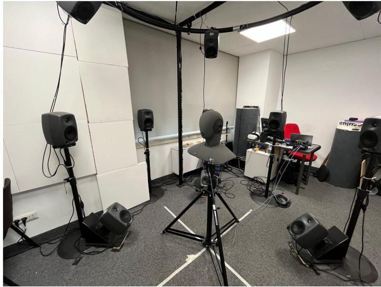
**Figure 3.12:** Dummy head simulator positioning for measuring procedures
