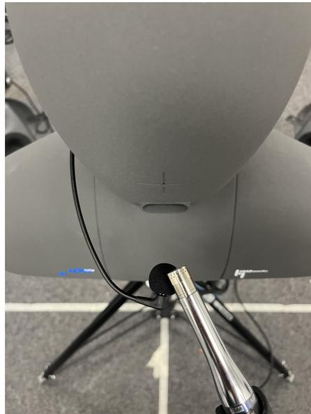
**Figure 3.10:** Positioning of the reference and head-worn microphones
