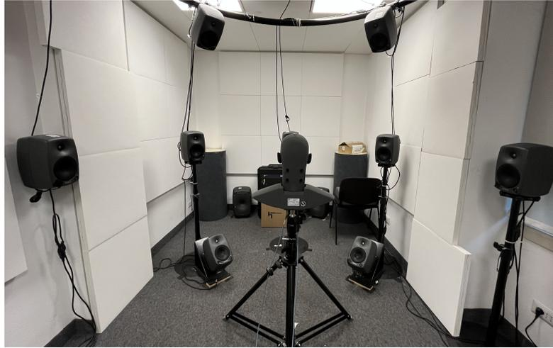
**Figure 3.11:** Dummy head simulator placed in the loudspeakers array
