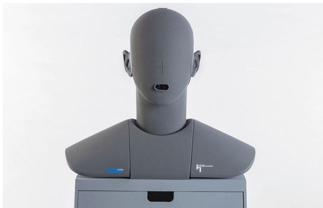
**Figure 2.7:** HEAD Acoustics - HMS II.3 LN HEC artificial head
