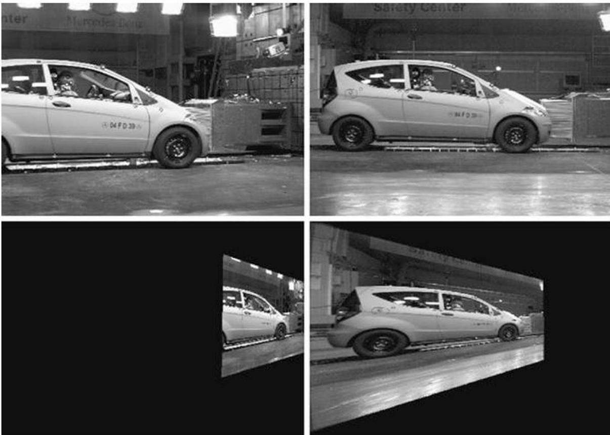
Figure 1 Top: Images recorded by two cameras with significant differences in extrinsic parameters and also differences in intrinsic parameters. Bottom: Two geometrically rectified images taken at different viewing locations by two cameras installed in a crash-test hall [6]
