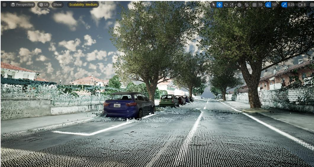
Fig. 4.8 The Mappano point cloud is combined with CARLA assets in Unreal Engine, creating an interactive simulation environment.
