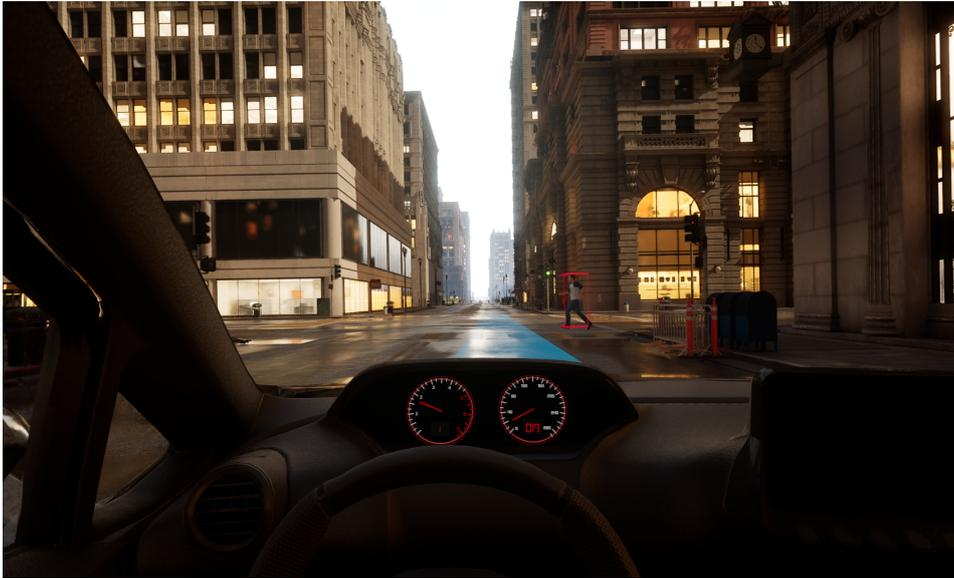
Fig. 7.4 The HUD interface highlights a detected hazard using a red bounding box, alerting the driver in real time.
