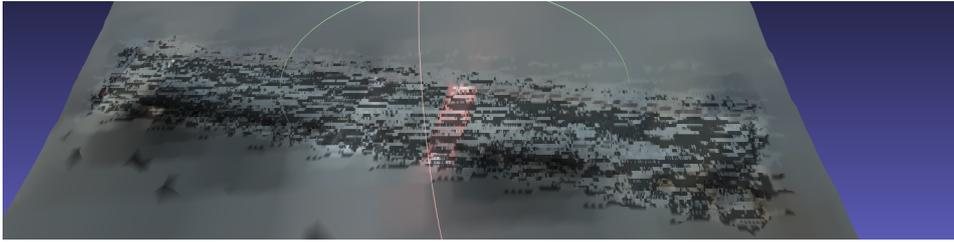
Fig. 4.4 Result of the Poisson mesh reconstruction algorithm applied in MeshLab, highlighting unwanted artifacts generated during the process.
