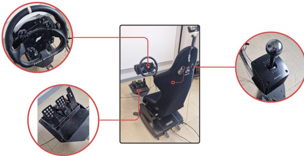
Fig. 6.1 The complete simulation setup featuring the Atomic A3 racing seat, highlighted Fanatec equipment including the steering wheel, pedals, and shifter, providing an immersive driving experience.
