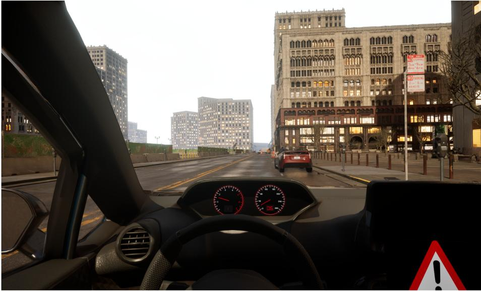
Fig. 7.2 The HDD interface marks a detected hazard with a triangular warning symbol on the navigation display.
