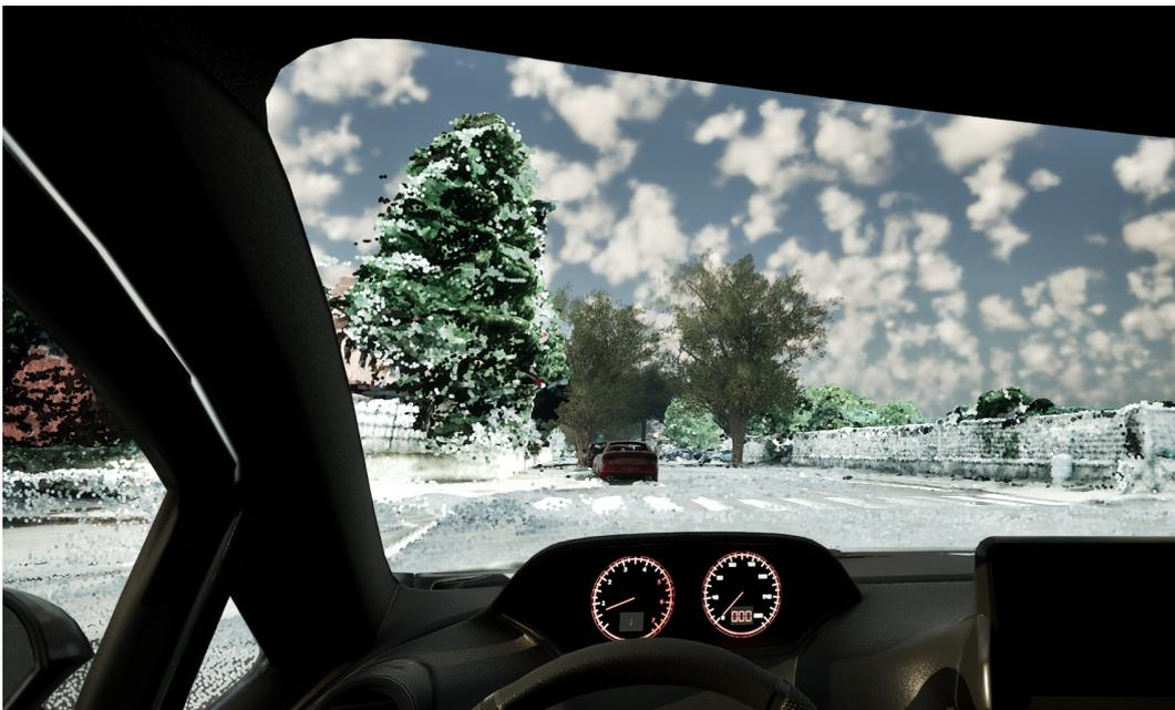
Fig. 4.9 The final Mappano map in CARLA integrates LiDAR point cloud data, CARLA assets, and OpenDrive information to create a navigable Digital Shadow simulation environment.
