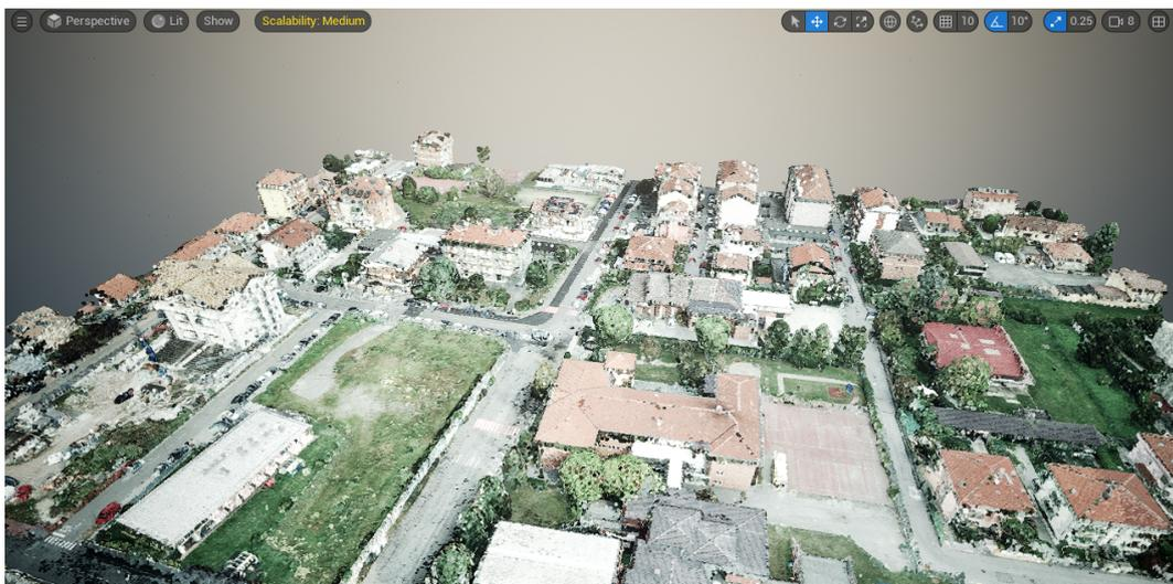
Fig. 4.6 The Mappano point cloud imported into Unreal Engine through the LiDAR Point Cloud Support plugin.
