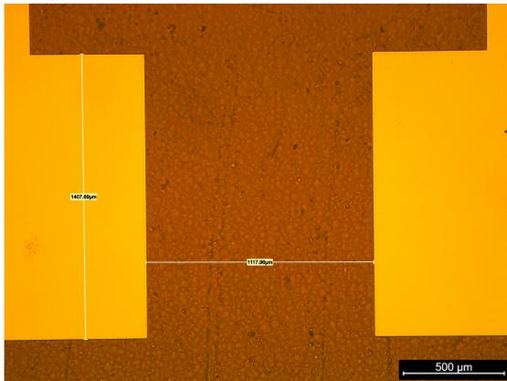
Figure 2.1: Microscope image of the gold electrodes at the end of lithographic process on polyimide substrate. Measured distance between the electrodes.
