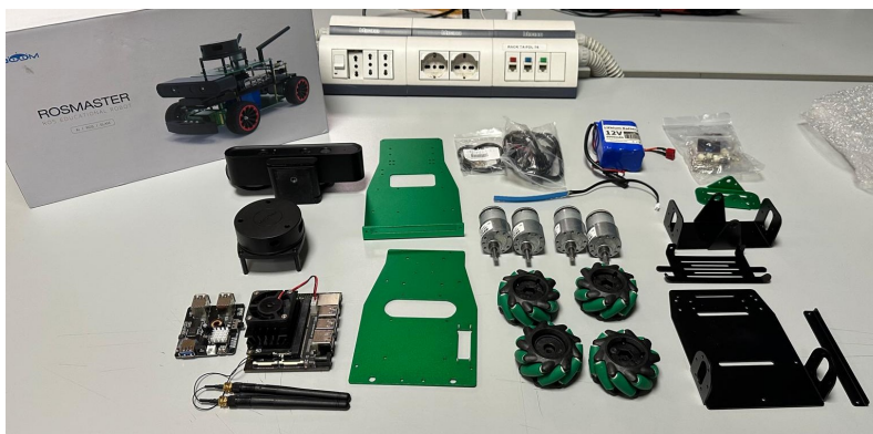
Figure 3.8: ROSMASTER X3 components
