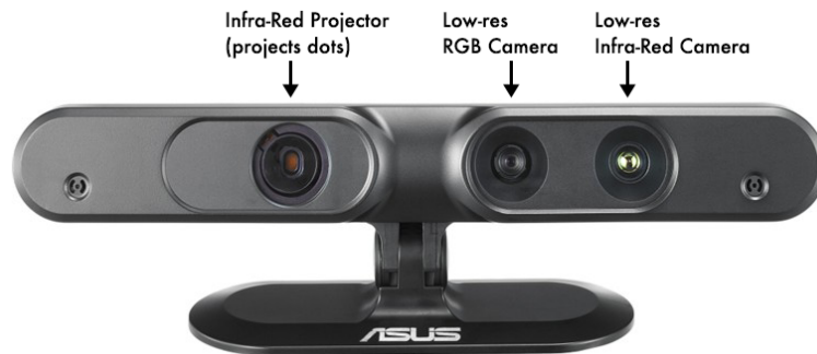
Figure 2.8: The components of a depth sensor
