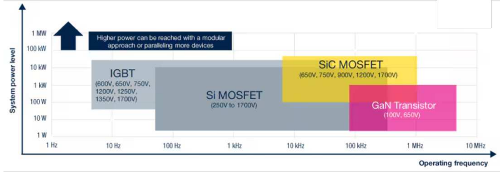
Figure 3.6: Switches technology selection based on power and frequency
