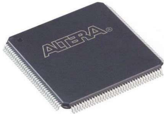
Figure 3.38: Altera MAX10 144QFP package.
