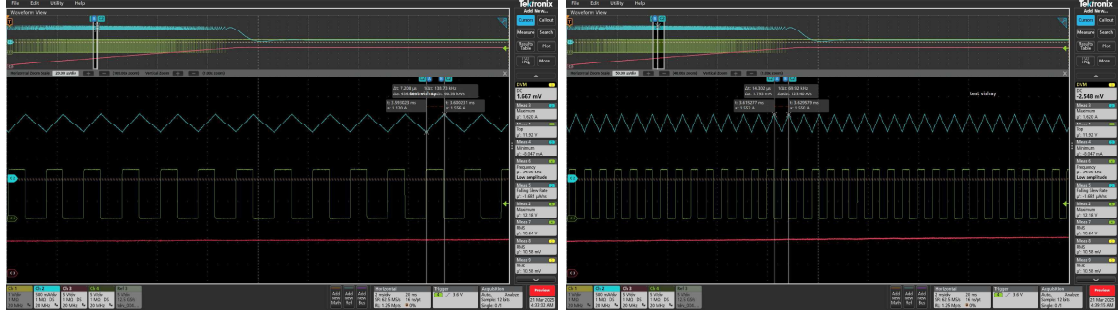
(a) Hysteresis thresholds measurement.
