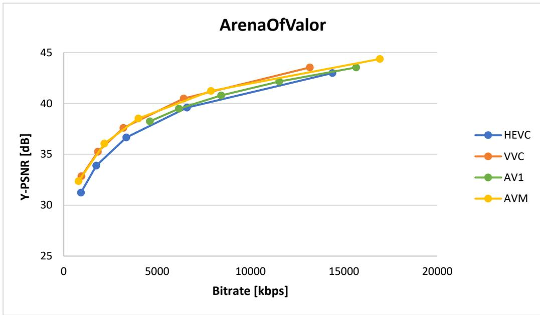
Figure 3.1: ArenaOfValor's Bitrate-PSNR graphic.
