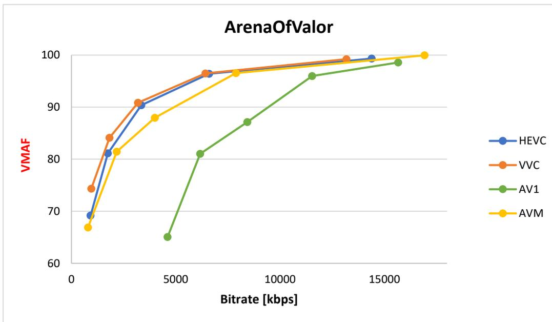
Figure 3.2: ArenaOfValor's Bitrate-VMAF graphic.
