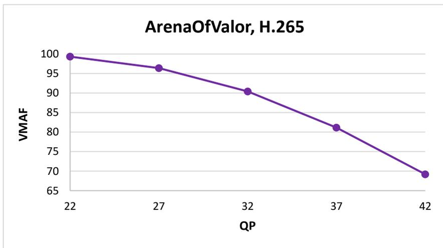
Figure 2.4: ArenaOfValor (HEVC), comparison between QP and VMAF.
