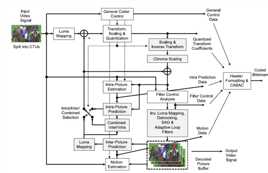
Figure 1.8: Typical VVC codec's path. [28]
