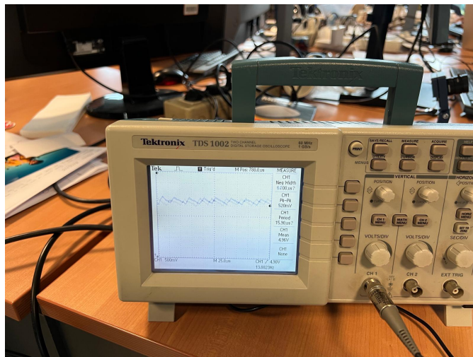
Figure 3.16: Ripple shown by the oscilloscope
