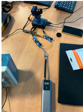
Figure 3.15: Test with the stepdown connected in parallel
