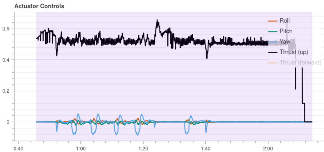
Figure 7.29: SIL normalized control input[12].
