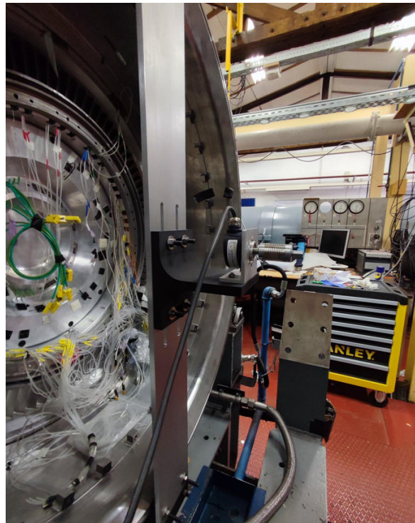
(b) Detail of the encoder mounted on its base, with emphasis on the flexible coupling. This component is key as the minor eccentricity on the real setup is nullified by it, allowing the testing sessions to proceed without any issues.
