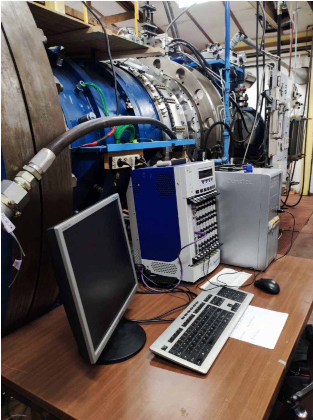
Figure 3.1: Detail of the data acquisition setup and the CT3 facility in the background. From the left to the right: Pc monitor, Genesis Tower, PC "Tuttec13".
