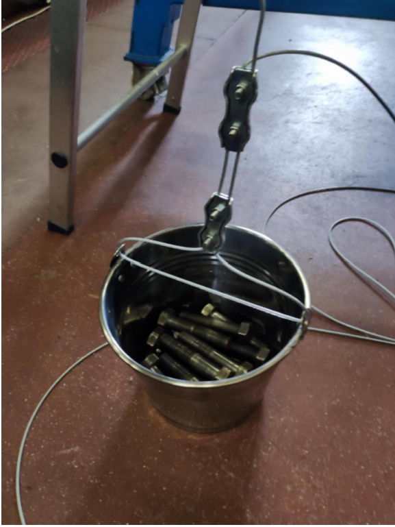
(a) The bucket used for generating the torque and its weight, M16 and M18 screws are used to generate the force necessary to move the rotor assembly.
