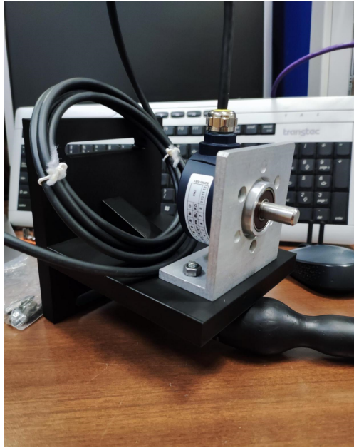
Figure 2.3: Encoder mounted on its base before being fixed on the final setup. In detail the encoder sensor is fixed on the "9202" [6] mounting bracket, the black component is the 3D printed "C3 - Encoder Base".
