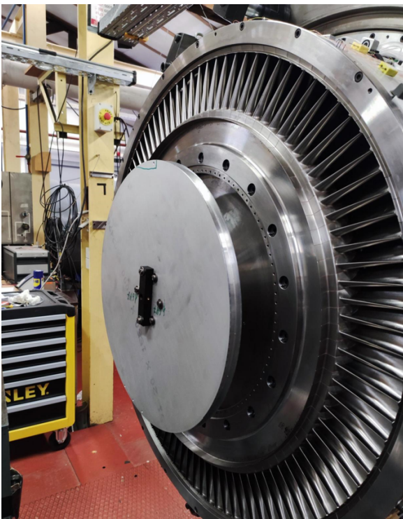
(a) Overview of the final aluminium disk.
