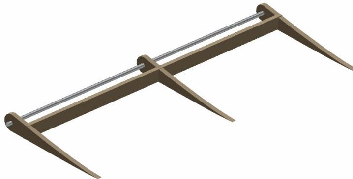
**Figure 2.13:** Control surface internal structure
