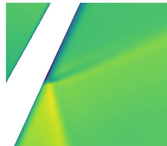
**Figure 5.7:** Shock-Boundary layer interaction
