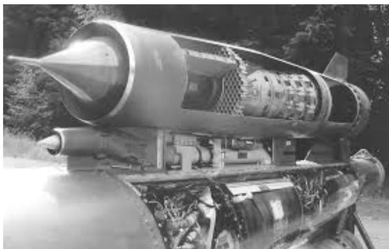
**Figure 1.6:** Oswatitsch intake mounted on a missile [15].
