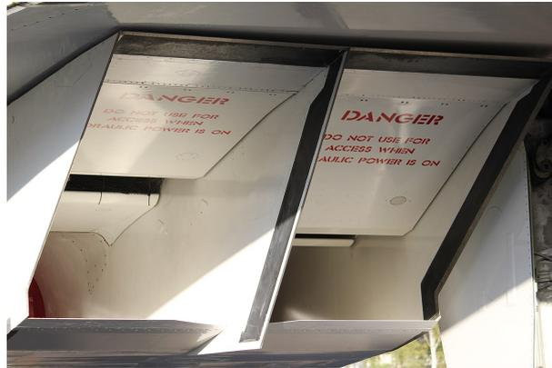
**Figure 1.5:** Prandtl-Meyer intake mounted on Concorde [12].
