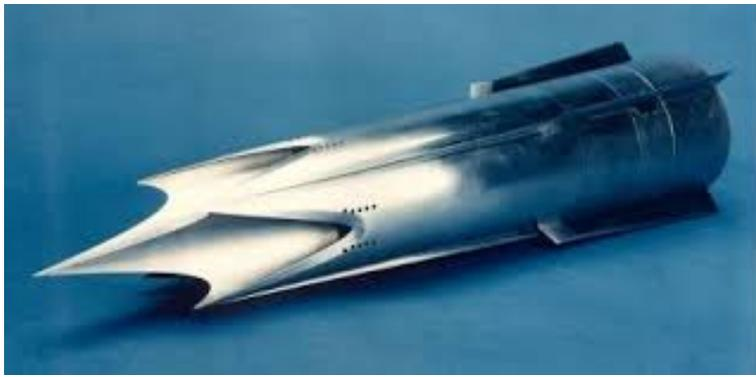
**Figure 1.7:** Four-module Busemann intake [18].
