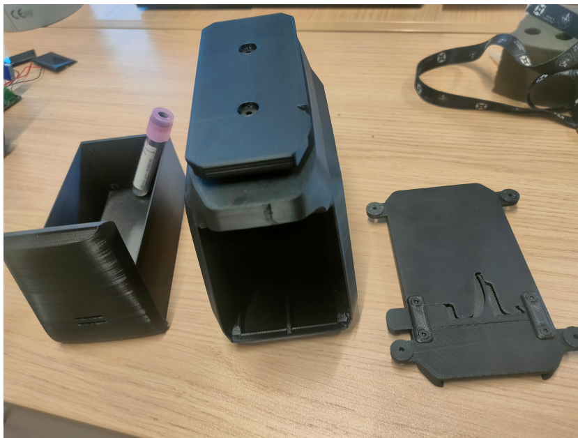
Figure 4.8: Capsule printed by LMA after slight adjustments
