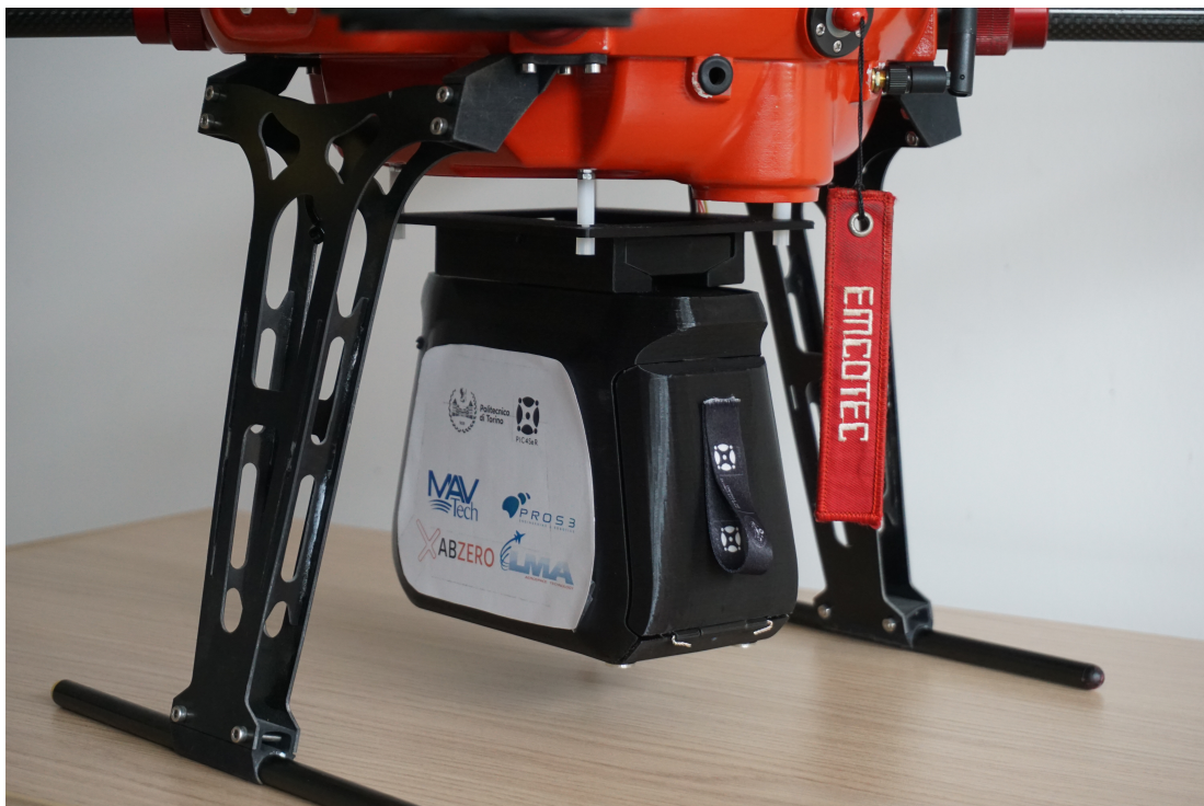
Figure 4.6: 3D printed mini capsule assembled and mounted under the drone
