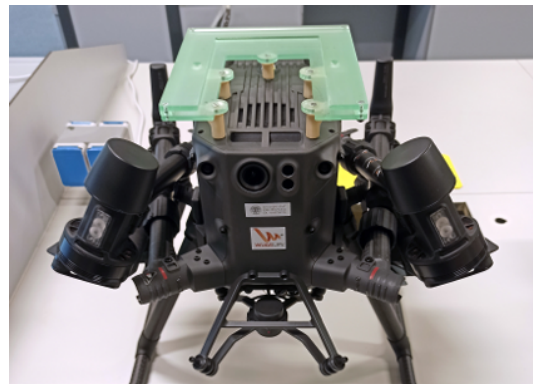
Figure 2.6: Quintanilla's DJI Matrice 300 RTK fitted with upper cargo bay
