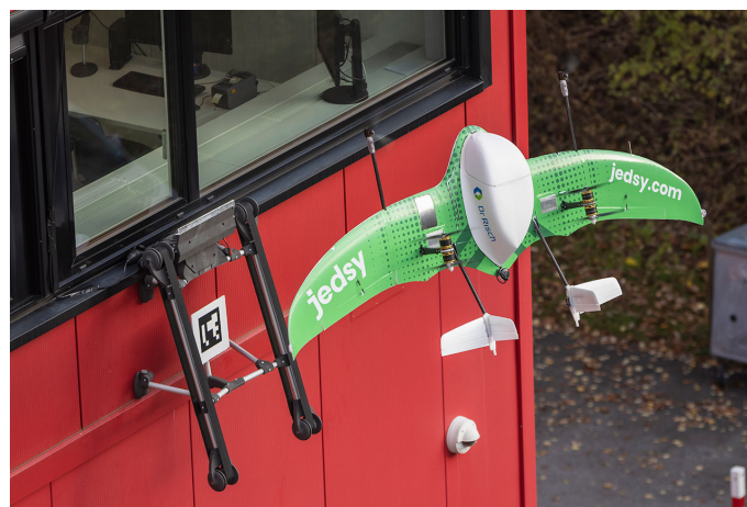
Figure 2.7: Jedsy drone that docks directly to a station anchored on windows
