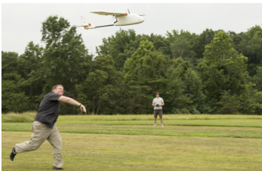
Figure 2.1: Amukele testing blood samples on a glided fixed-wing drone
