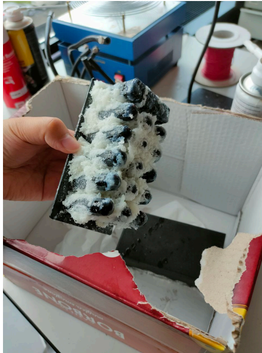
Figure 4.11: Direct contact of the polyurethane foam with a PLA expansion chamber results disastrous
