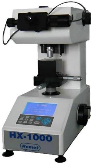
Figura 7.14: Microdurometro Remet HX 1000 [56]
