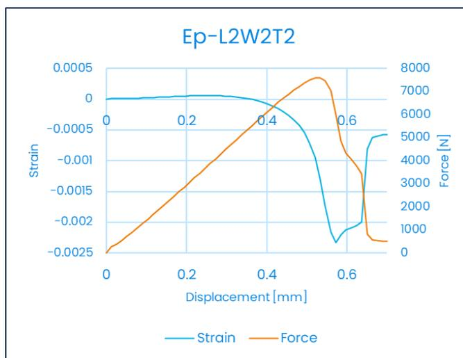
Figure 7.40: Strain-displacement and force-displacement curves for numerical result of Ep-L2W2T2
