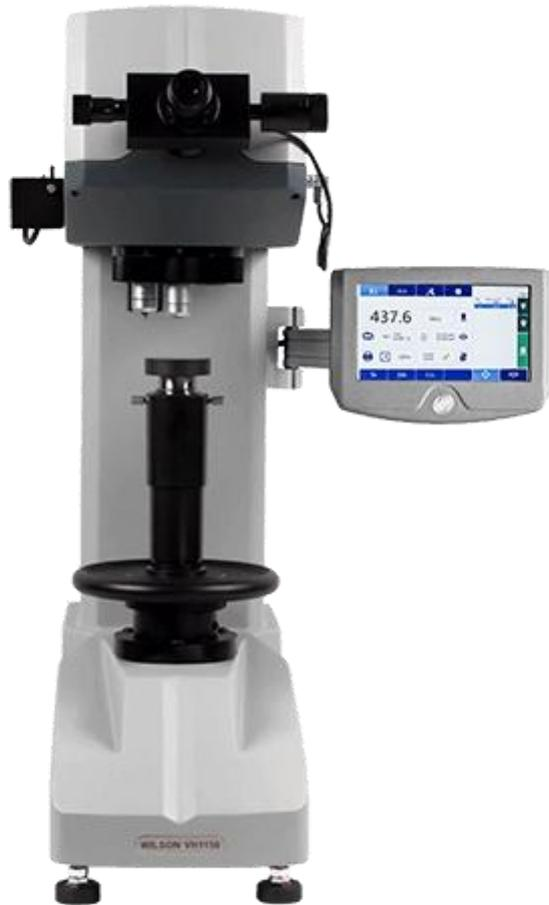
Figure 2.10: Microhardness tester Wilson VH1150
