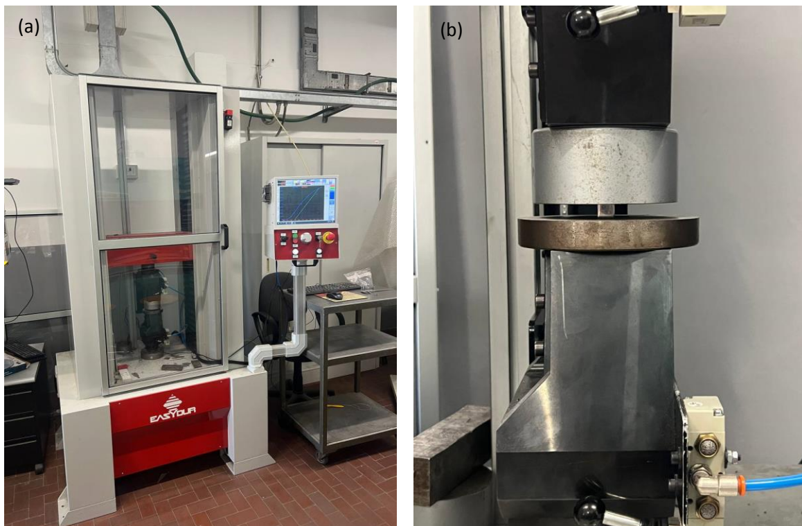
Figure 39: (a) EASYOUR compression test machine , (b) upper and lower test plates
