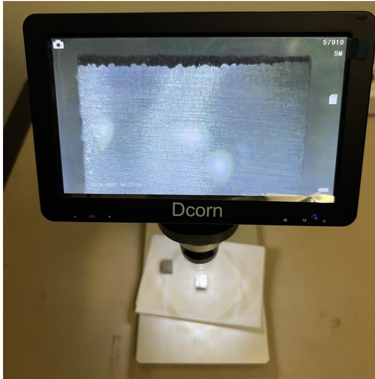
Figure 31: using microscope for assessing the visibility of the grinding lines
