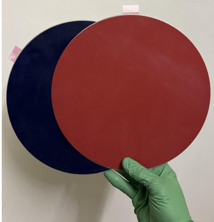
Figure 33: Polishing pads with 3-micron(blue) and 1-micron(pink) grit sizes were used for polishing the samples
