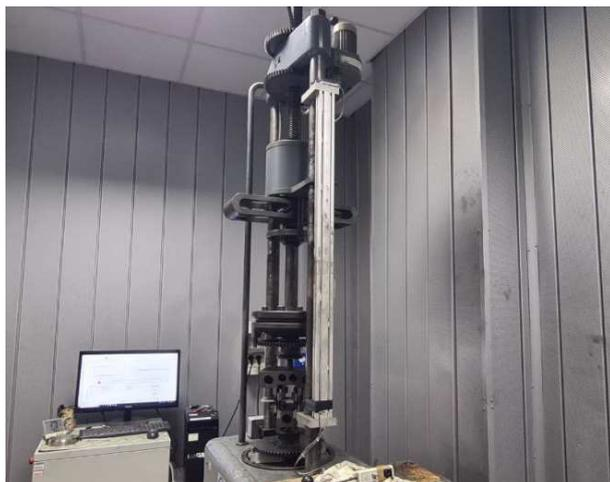
Figure 4.6: Vibroforo Amsler HPF 100
