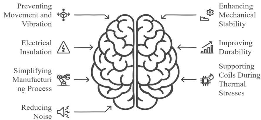
Figure 35 The Role of Lacing in Stators
