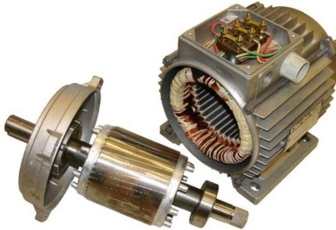
*Figure 34 Rotor and Stator [v]*
