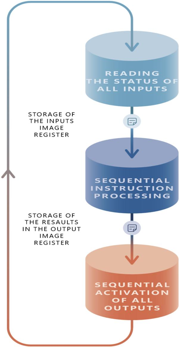
Figure 6 PLC operation diagram
