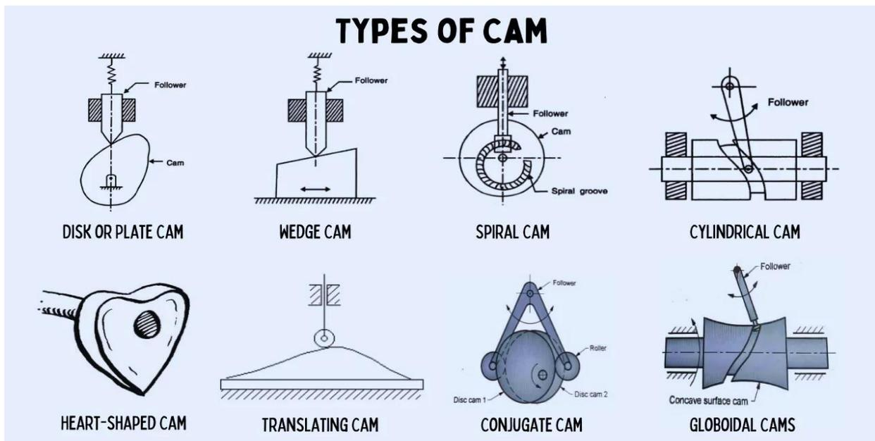
Figure 20 Different Types of CAMs [p]
