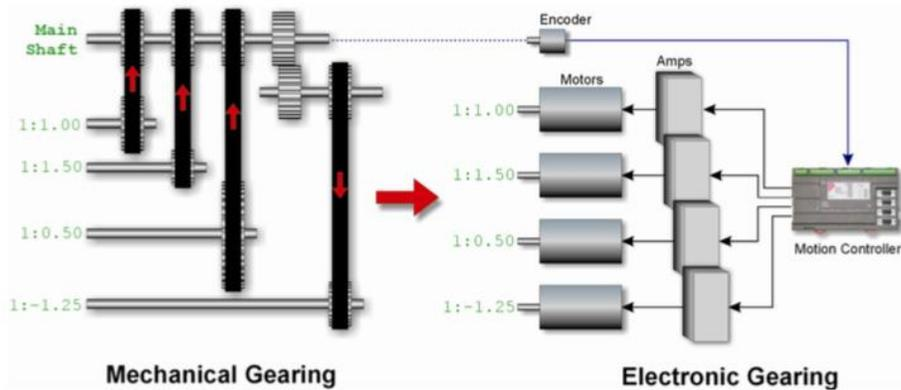
Figure 9 Electronic Gearing Vs Mechanical Gearing [g]
