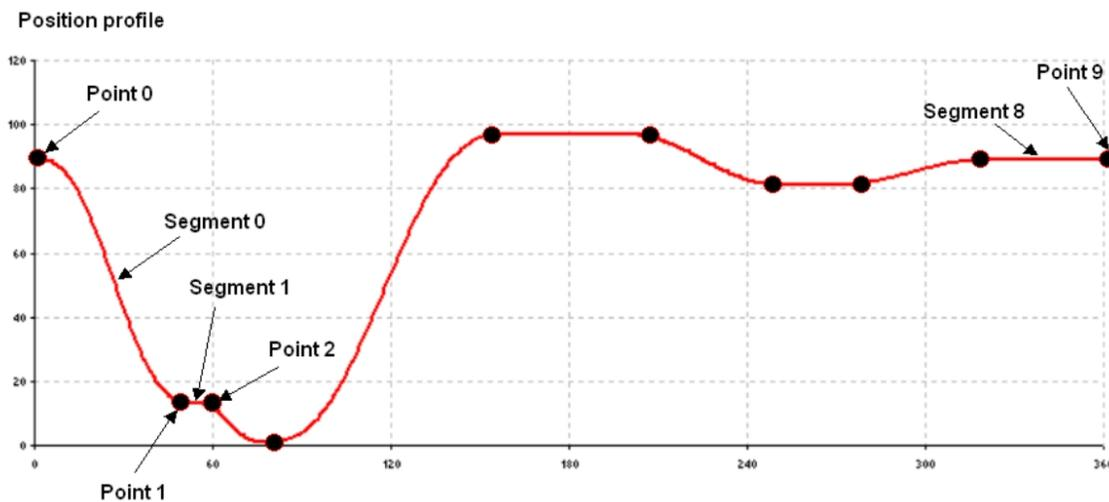
Figure 24 Cam disk consisting of several elements [s]
