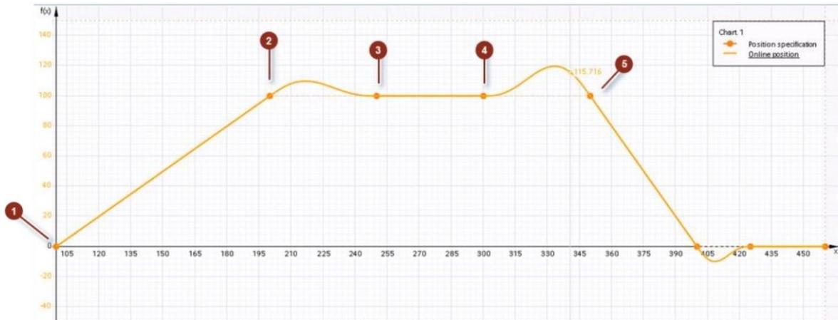
Figure 26 Cam disk with 8 points created by LCamHdl\_CreateCamBasic [s]
