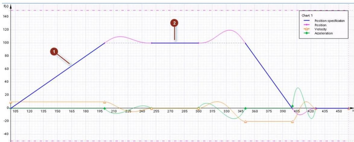
Figure 28 Cam disk with 4 segments created with LCamHdl\_CreateCamAdvanced [s]
