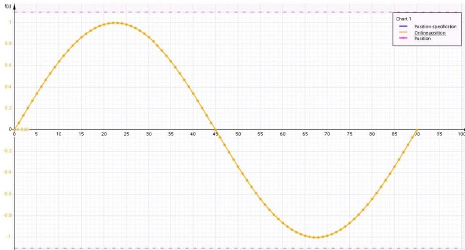
Figure 29 Cam disk example (interpolation mode C splines) created by [29]
