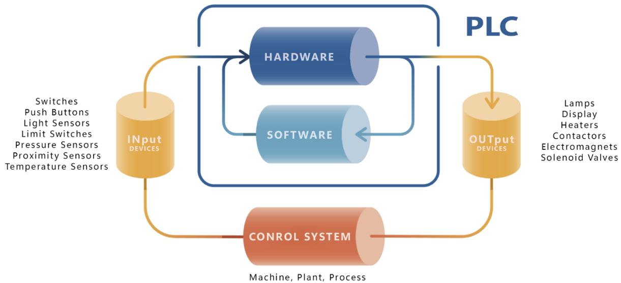
Figure 4 Hardware and software scheme of the PLC
