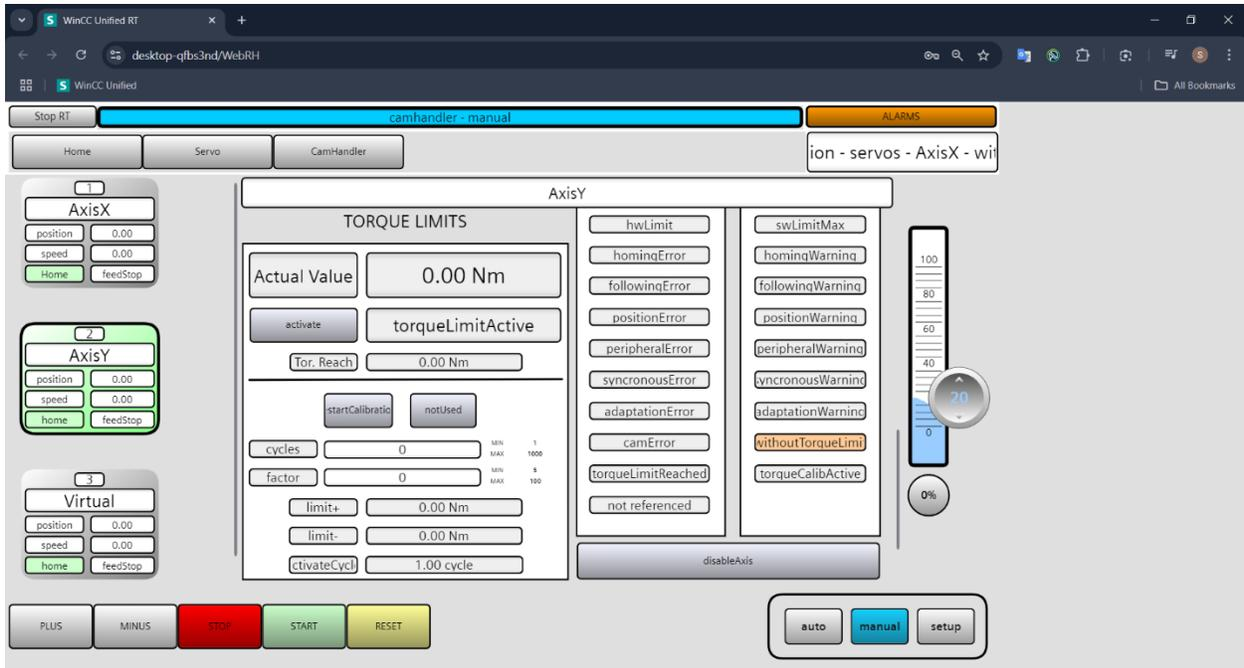
Figure 53 Torque Limits
