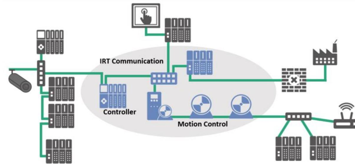
Figure 5 Example of the PROFINET connections [e]
