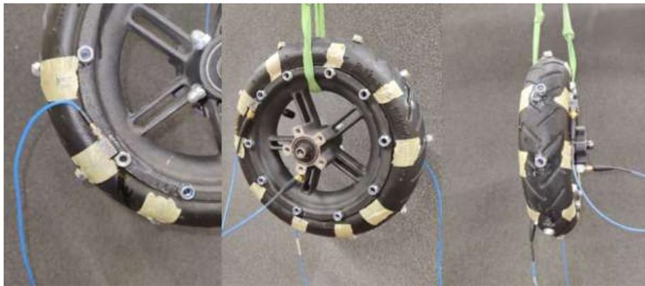
*Figure 3. 12 Tyre setup for Experimental Modal Analysis*
