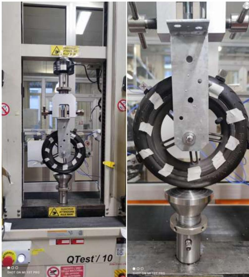
Figure 3. 1 Experimental setup of tyre on MTS machine for radial stiffness evaluation
