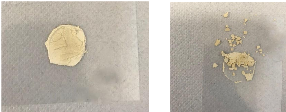
Figure 3. 2 The BZCY sample with 70%wt solid load, 2%wt dispersant, 5%wt plasticizer
