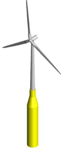
Figure 5.9: Spar platform. Adapted from [37].
